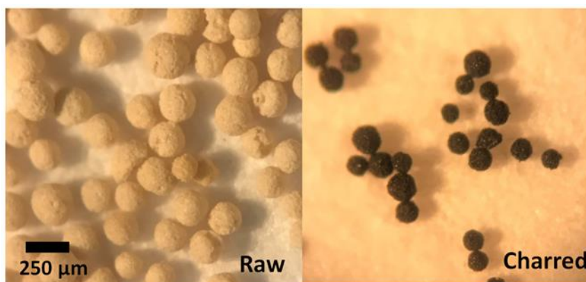
Fig. 2.1. An example of switchgrass particles in raw and charred condition observed under an optical microscope.
