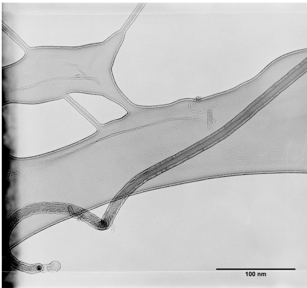
Figure 69: Block nitrogen doped nanotube demonstrating herringbone structure. In this instance the pristine section was grown prior to the nitrogen doped section, as indicated by the direction of the herringbone structure.
