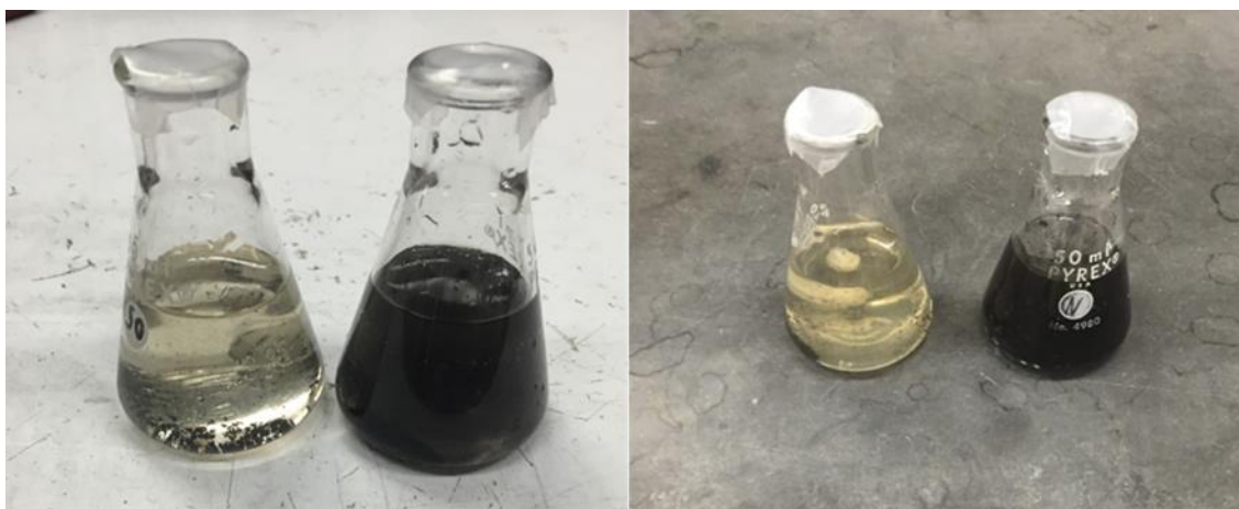
Figure 19: Pristine and Nitrogen doped nanotubes dispersed in water with polyacrylic acid after five minutes (Left) and 1 week (Right) showing stability of the system.
