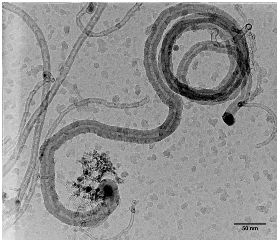
Figure 67: TEM image of a nanotube showing a catalyst particle at each end. The lack of bamboo or herringbone structure near either particle indicates both sides may have been available for growth during the ethylene growth phase.
