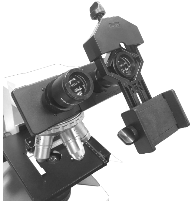
Figure 4: Cell cam mount. This contraption allows you to easily take pictures with your cell phone.
