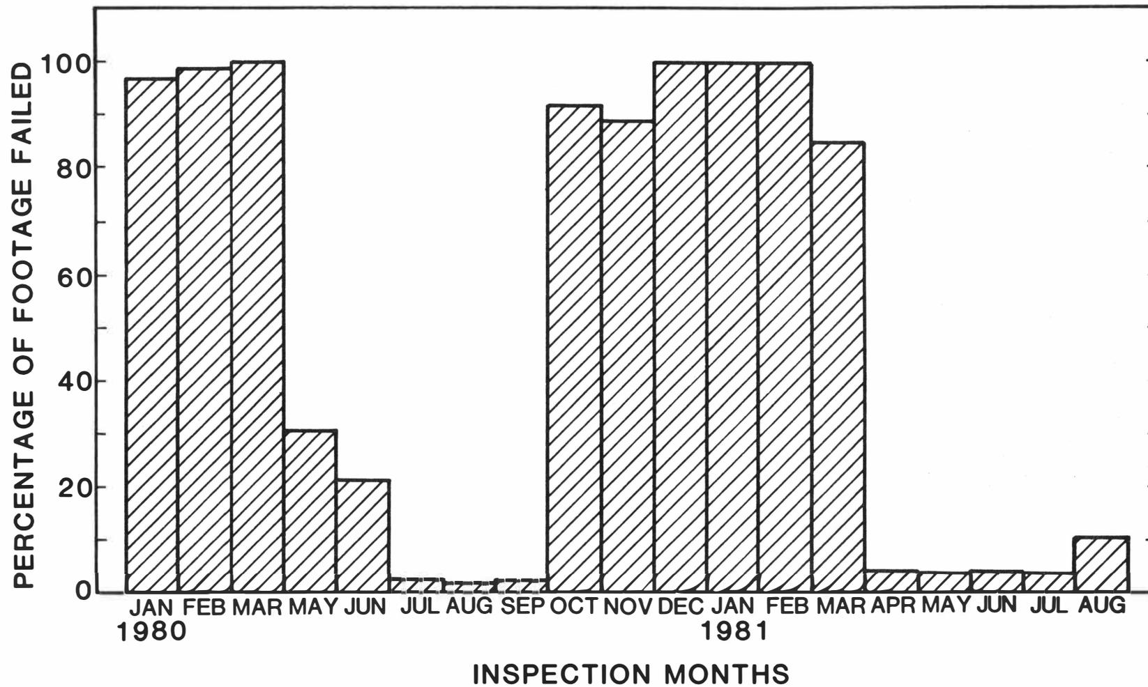
Figure 16. Field Performance of CRS-2 Sealant
