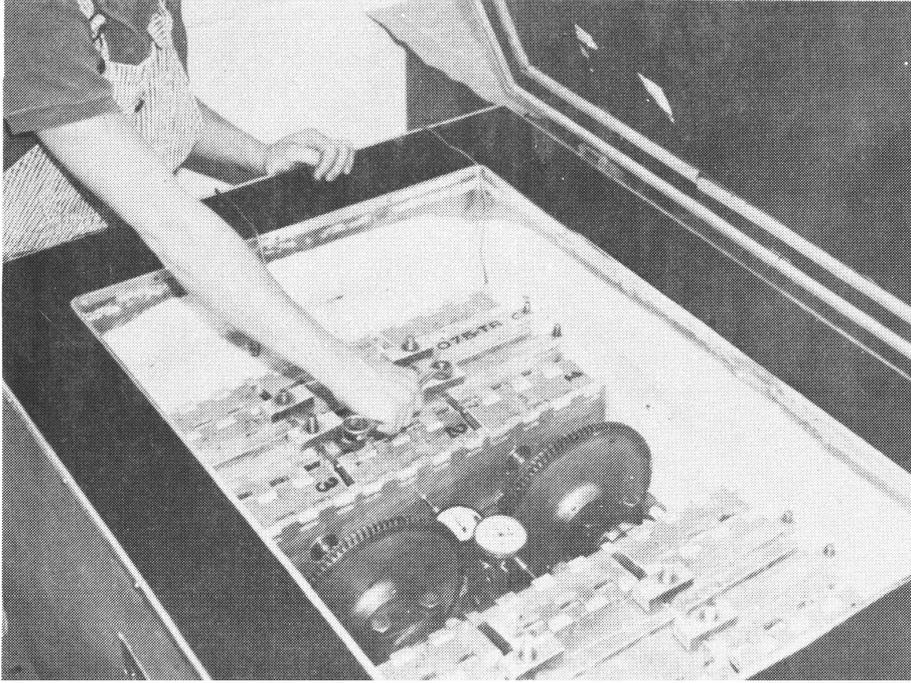
Figure 1. Bond-Ductility Machine with Six Sealant Specimens Being Clamped in Place for Testing
