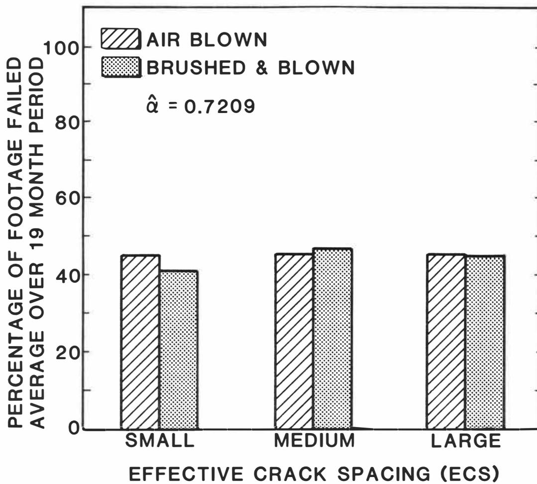
Figure 15. Interaction of ECS and Crack Pretreatment for 85-100 Pen AC Sealant
