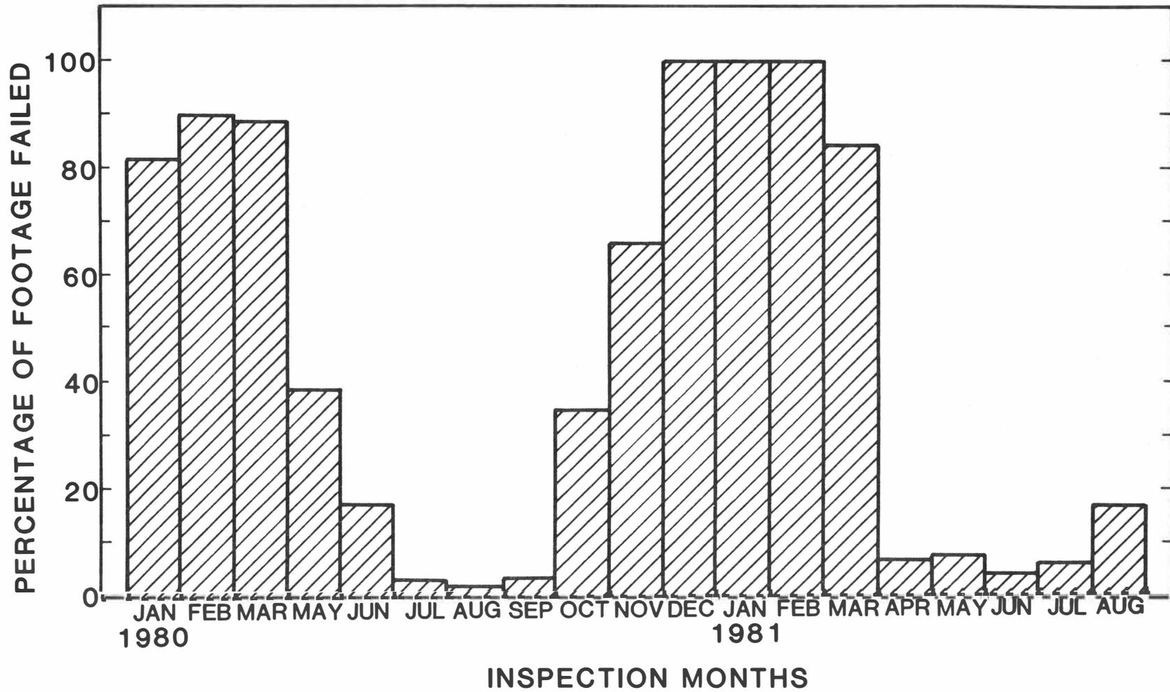
Figure 11. Field Performance of 85-100 Pen AC Sealant
