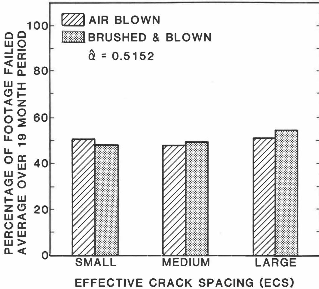
Figure 18. Interaction of ECS and Crack Pretreatment for CRS-2 Sealant
