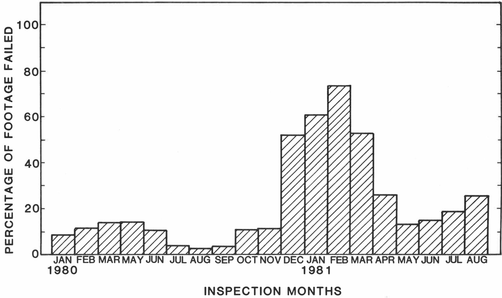
Figure 21. Field Performance of MSLV Sealant
