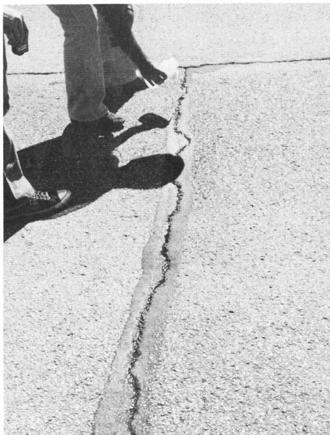
Figure 8. Testing Sealant Failures with Water
