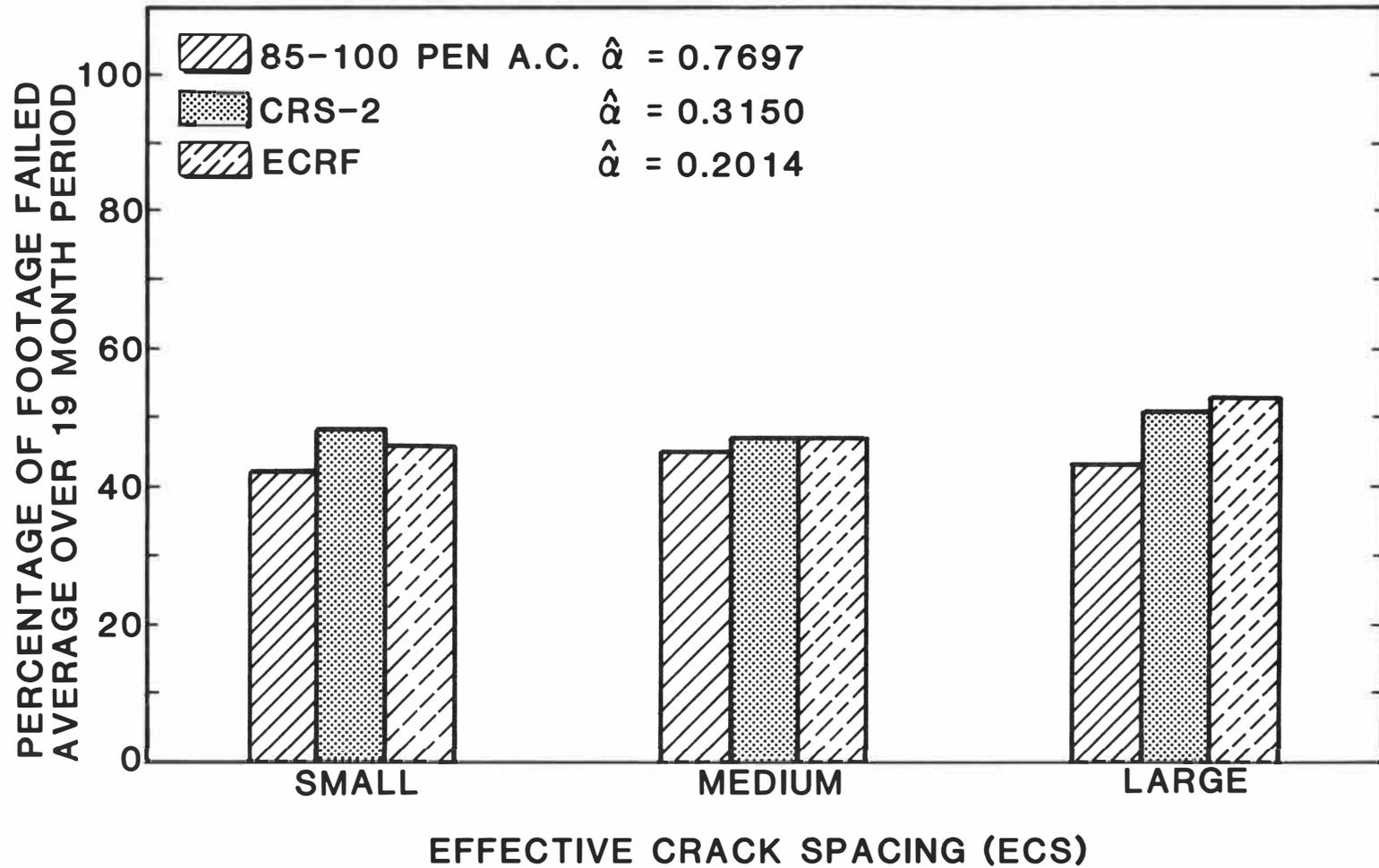
Figure 13. Percent of Sealed Crack Failure Vs. ECS for 85-100 Pen AC, CRS-2, and ECRF Sealants
