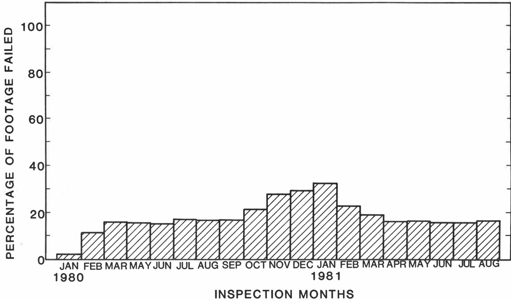
Figure 27. Field Performance of SOFS Sealant
