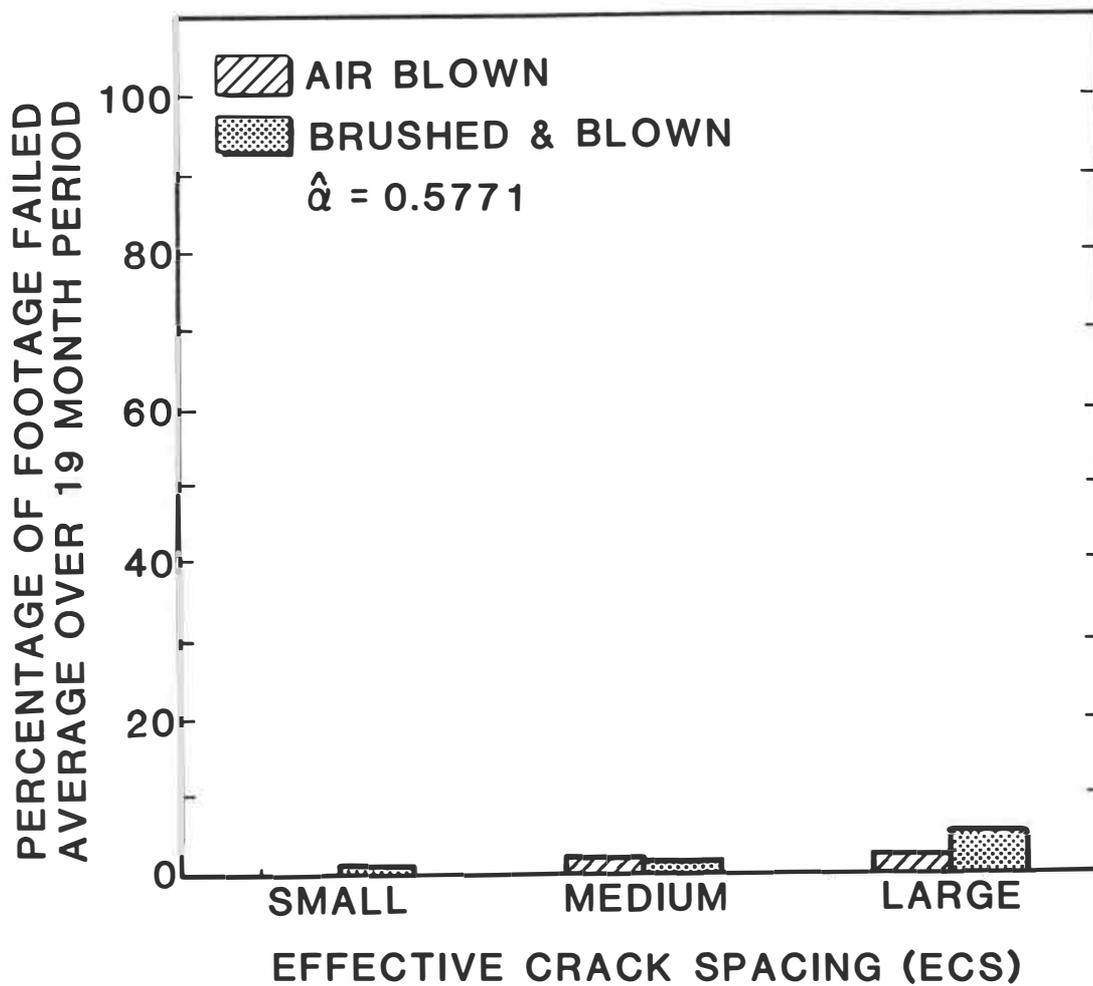
Figure 31. Interaction of ECS and Crack Pretreatment for HARS Sealant
