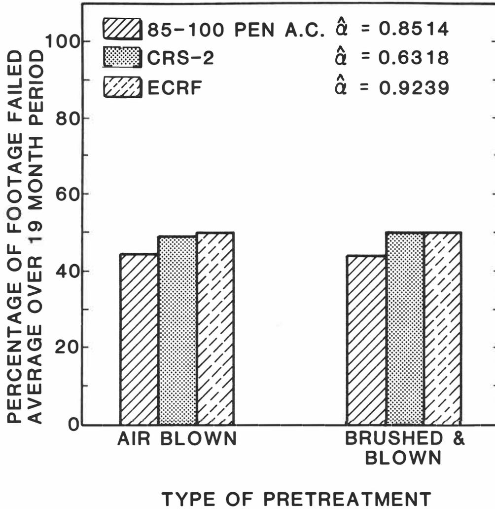
Figure 14. Percent of Sealed Crack Failure Vs. Crack Pretreatment for 85-100 Pen AC CRS-2, and ECRF Sealants
