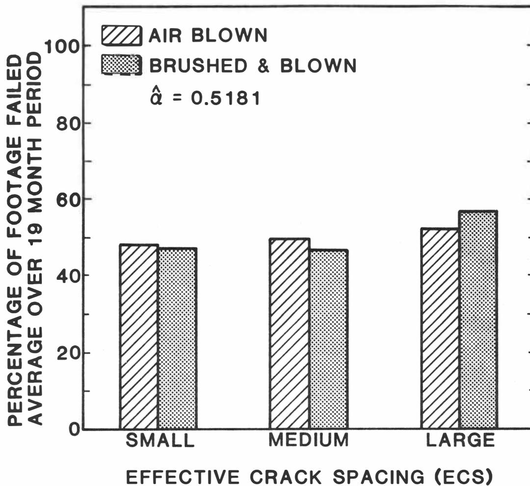
Figure 20. Interaction of ECS and Crack Pretreatment for ECRF Sealant
