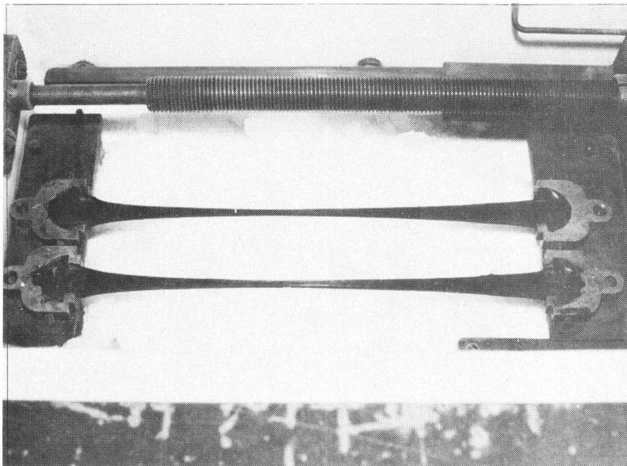
Figure 26. Elongation of SOFS Sealant Specimens in Modified Ductility Test
