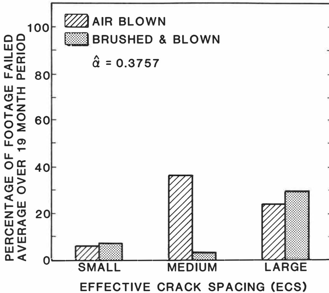
Figure 29. Interaction of ECS and Crack Pretreatment for SOFS Sealant
