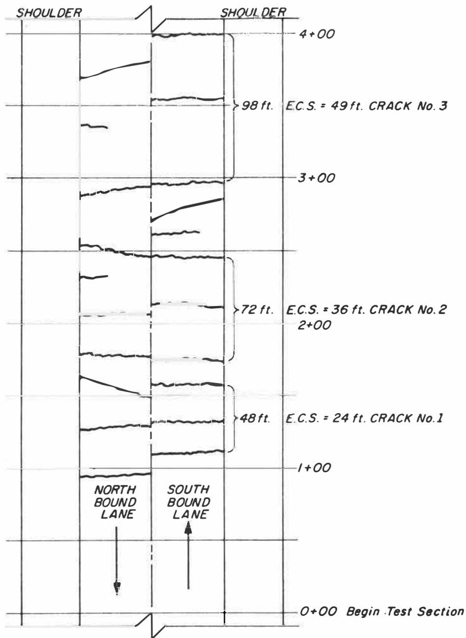
Figure 3. Crack Survey Data Sheet
