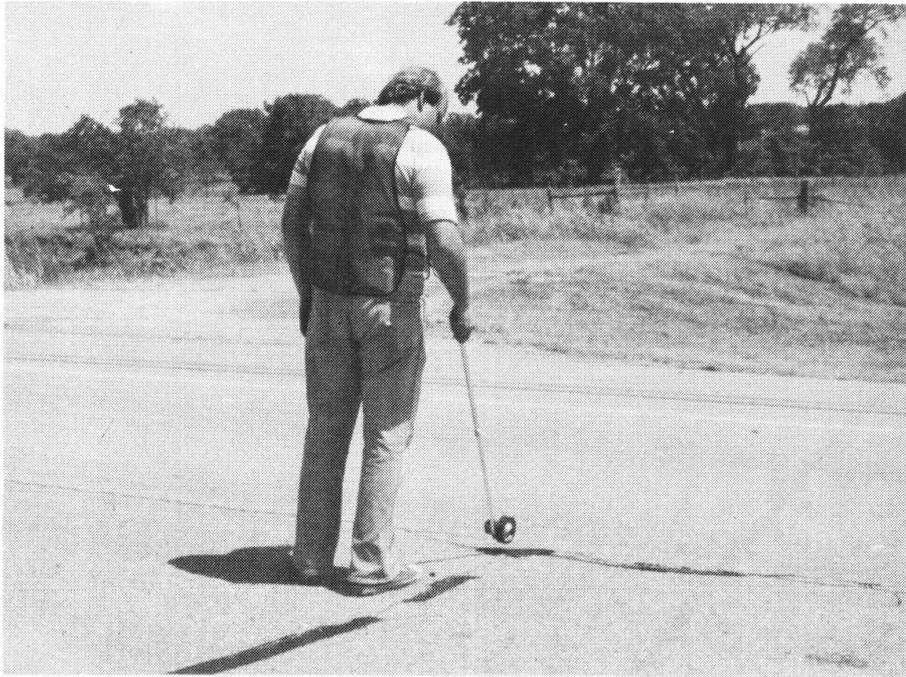
Figure 9. Measuring Failed Length of a Sealed Crack
