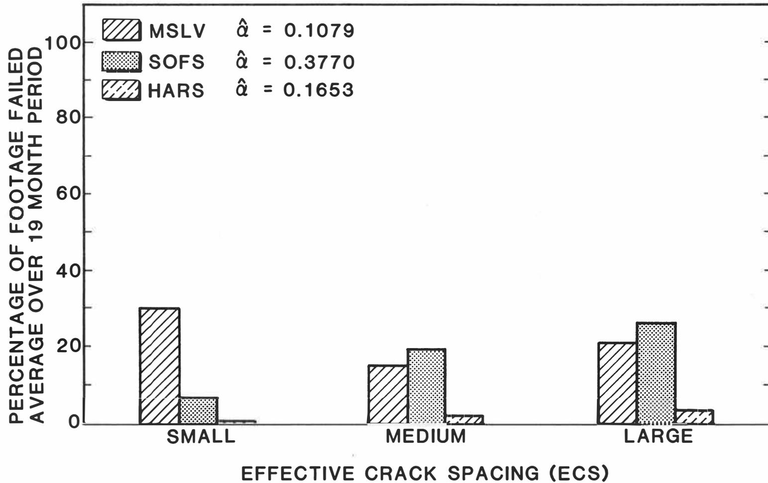
Figure 23. Percent of Sealed Crack Failure Vs. ECS for MSLV, SOFS, and HARS Sealants
