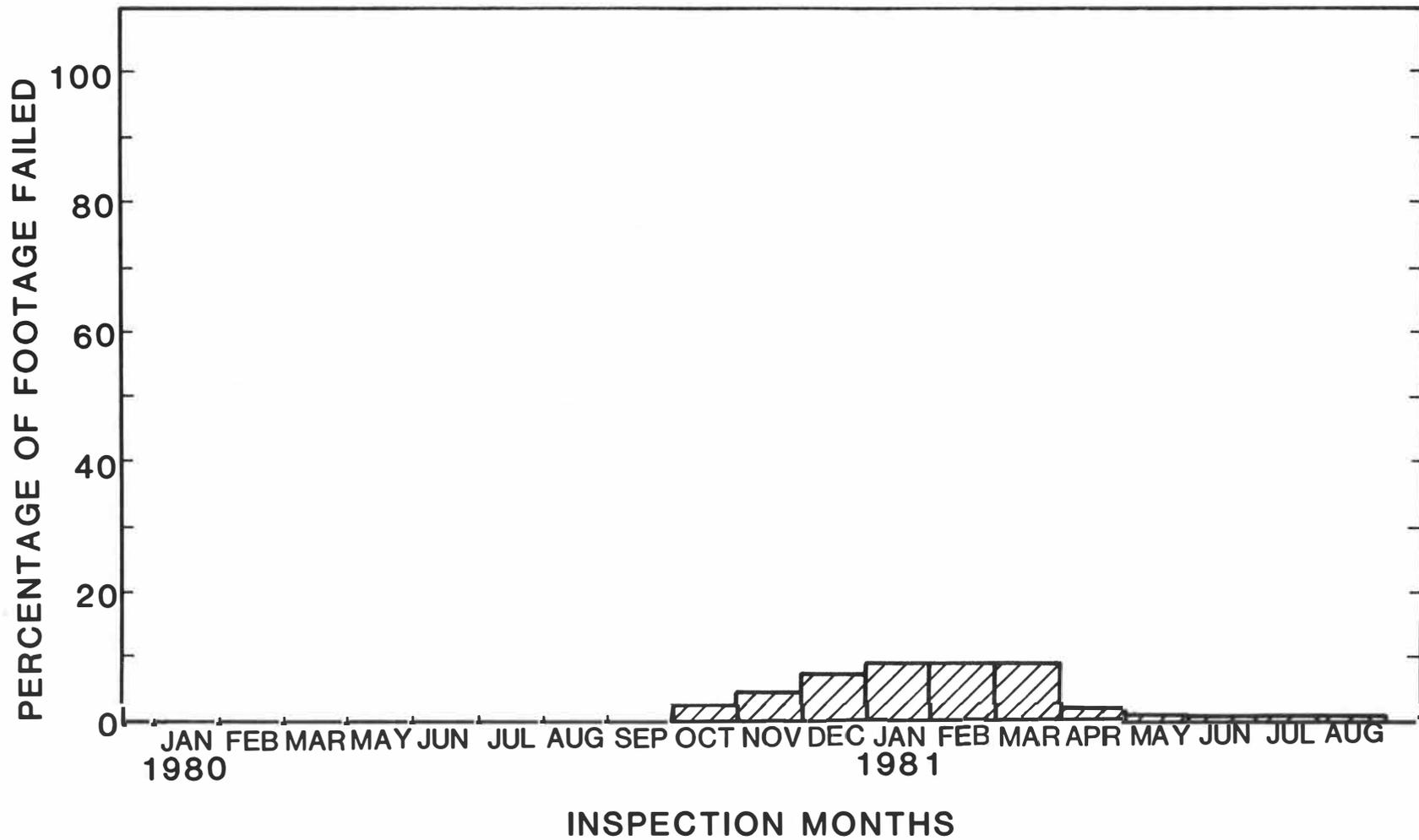
Figure 30. Field Performance of HARS Sealant
