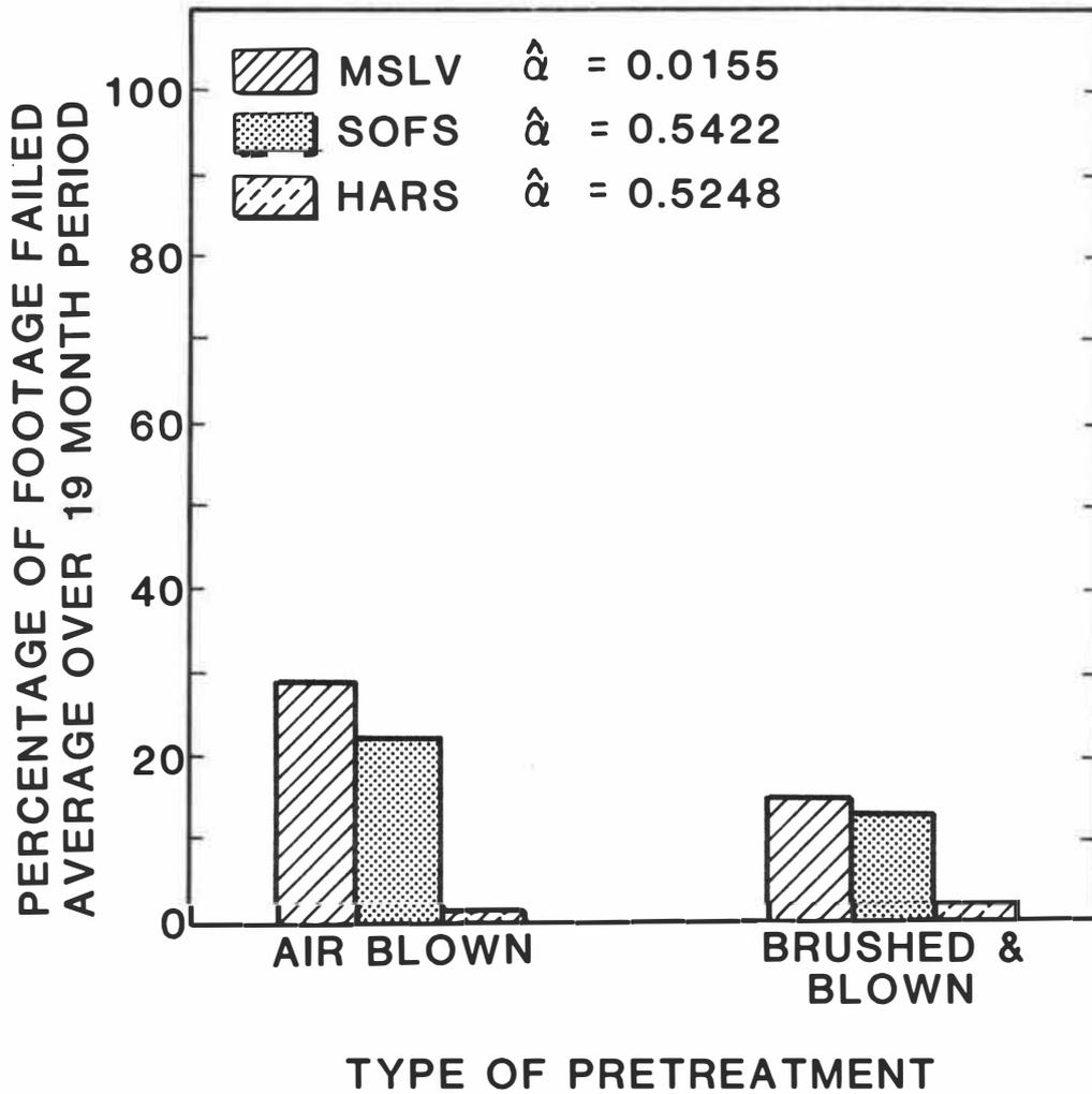
Figure 24. Percent of Sealed Crack Failure Vs. Crack Pretreatment for MSLV, SOFS, and HARS Sealants
