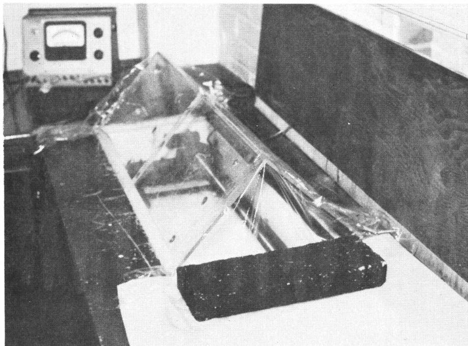
Figure 2. Modified Ductility Test Chamber
