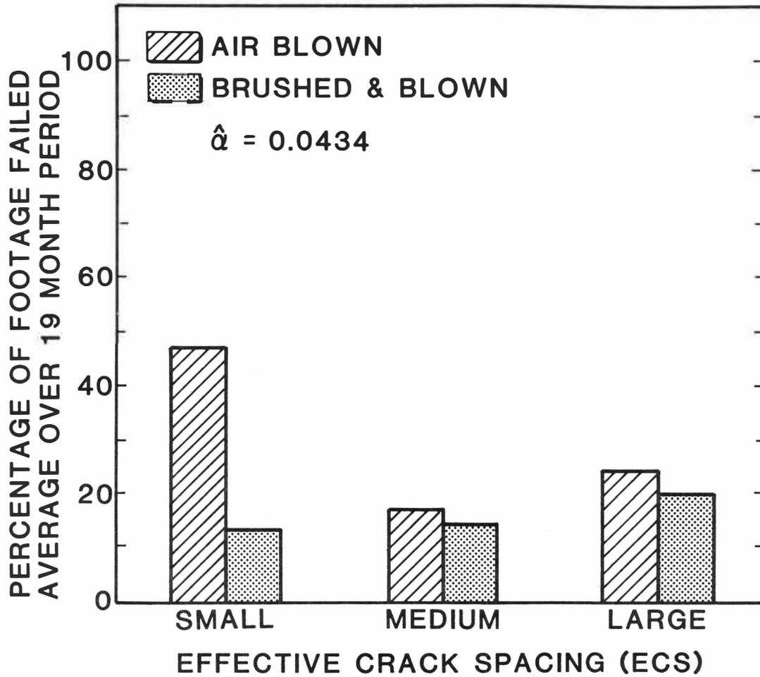
Figure 25. Interaction of ECS and Crack Pretreatment for MSLV Sealant
