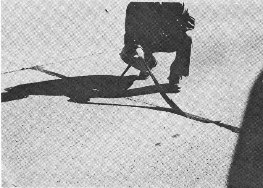
Figure 28. Rubber-Band Type Failure of SOFS Sealant
