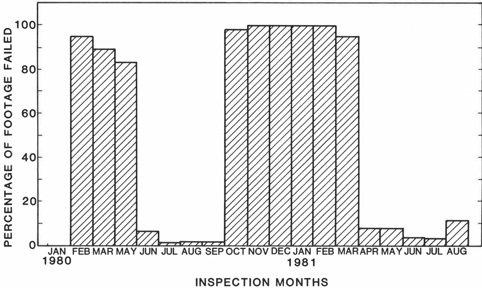
Figure 19. Field Performance of ECRF Sealant
