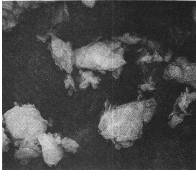
Figure 5.15: Electron micrograph of shale 35.
