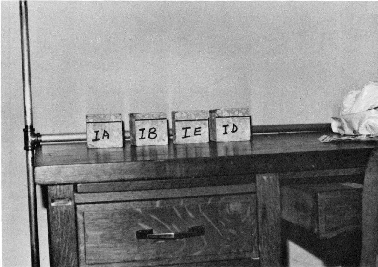
Figure 1.4A Impregnated Slabs Showing Polymer Depth.
