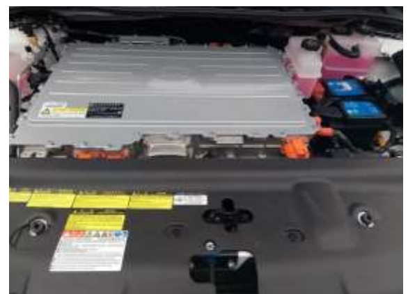
Figure 5. A typical battery found in an electric vehicle. By DKMcLaren Licensed By CC BY-SA 4.0
