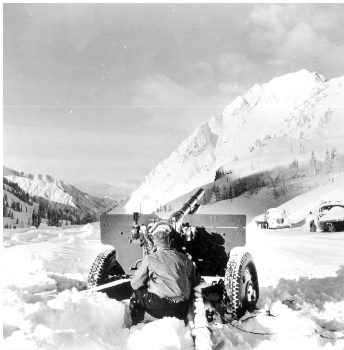
Figure 10. Photo taken by Ed LaChapelle of 75mm used in avalanche control at Alta (1956). Courtesy of U.S. Forest Service Intermountain Regional Office, Wasatch National Forest Photo Collection.
