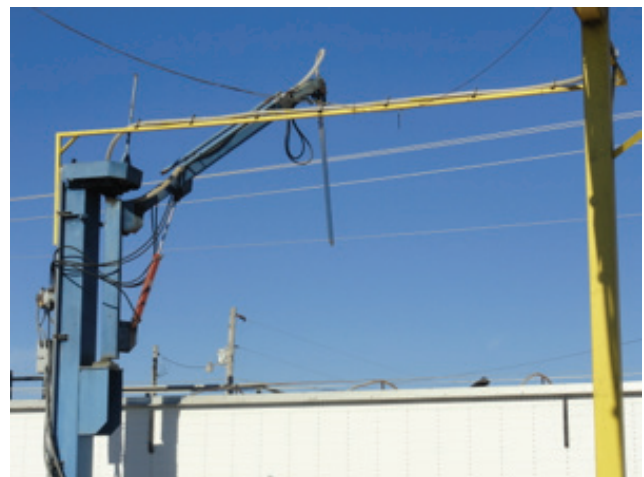
Figure 1. Automatic sampler ready to gather a sample from an incoming grain truck.
