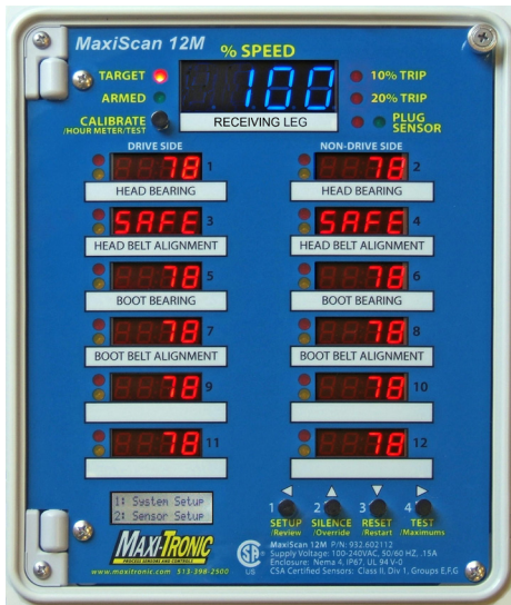
Figure 11. Example of a bearing temperature and belt alignment readout panel.
