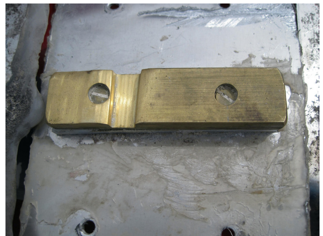
Figure 6: Worn belt alignment block.
