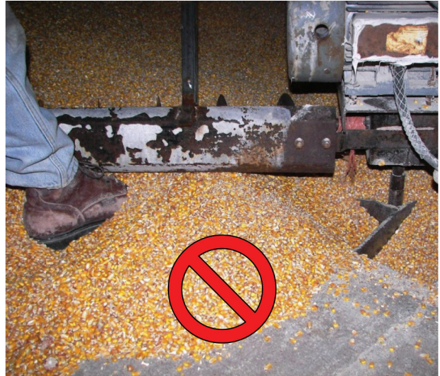
Figure 15. Moving grain around the sweep auger with a foot is an unsafe practice.
