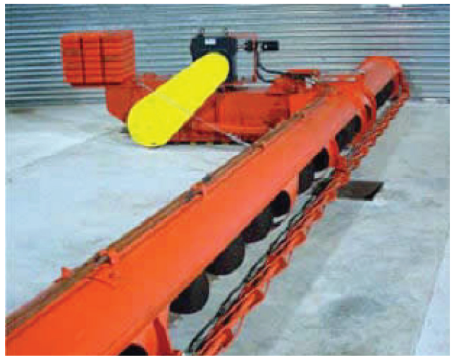
Figure 8. Sweep auger with acceptable guarding.
