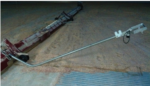
Figure 10. “Dead man” control handle for sweep auger.
