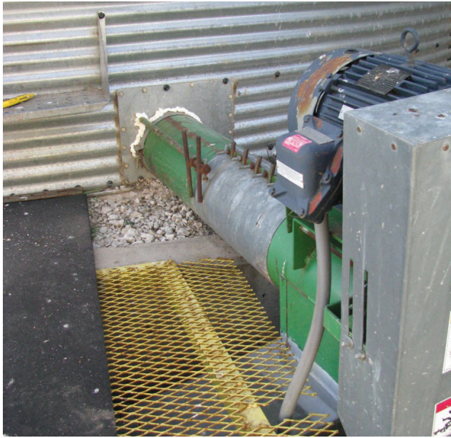
Figure 14. Unloading auger with permanent sealing on bin penetration and temporary sealing on slide gate push rod opening.
