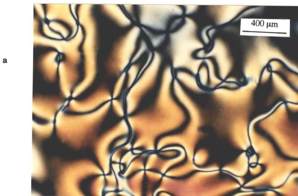
Figure 20. Polarizing micrographs of the textures of 4-(10-undecylenyloxy)benzoic acid: (a) obtained on heating to 125 °C in nematic phase; (b) obtained on cooling to 80 °C in the smectic C ( S_C ) phase.
