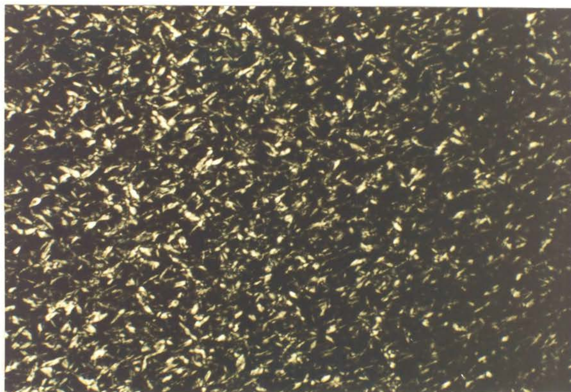
Figure 17. Polarizing micrographs of the hexamine 2 complex of \text{Pd}(\text{O}_2\text{CCH}_3)_2 (1:1). (a) before heating, at 20 °C; (b) heated to 70 °C.
