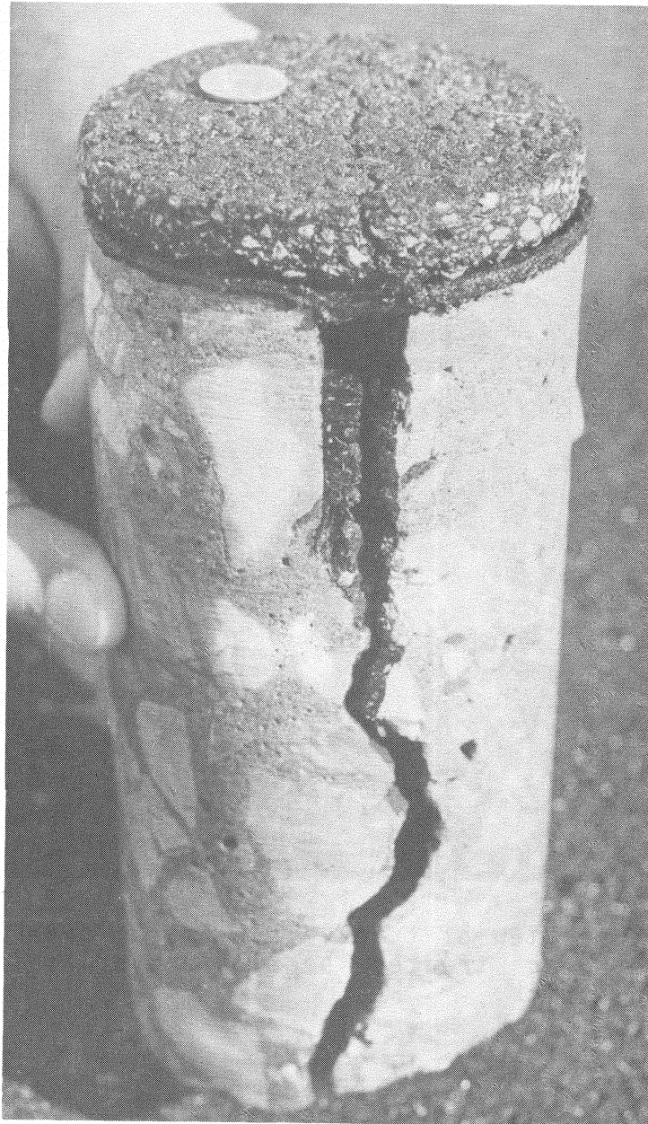
Figure 15. Core taken over the reflected transverse crack in the Petrotac section - overlay less than 1 inch thick. Note the "sealed" joint.
