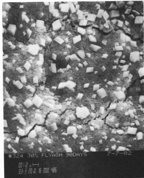
Figure 5.25 30% Fly Ash Concrete @90 days (3000X)
