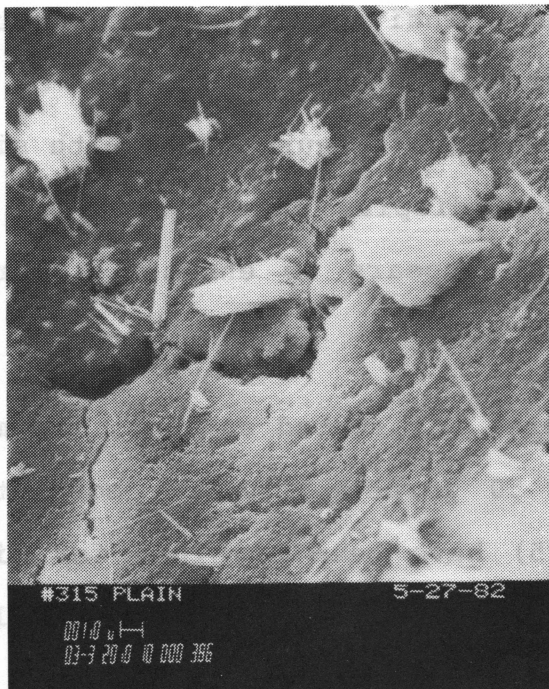
Figure 5.16 Plain P.C. Concrete @ 28 days (3000X)
