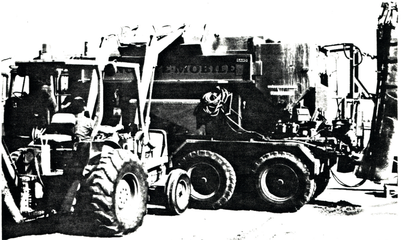
Figure 4. Concrete-Mobile was loaded with the dried aggregate.
