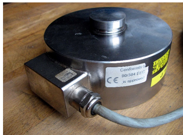
Figure 4.37: Compression style strain gauge load cell. © Jindřich Běťák. Used under CC BY-SA license: https://en.wikipedia.org/wiki/Load_cell#/media/File:Silomer_100kN.jpg
