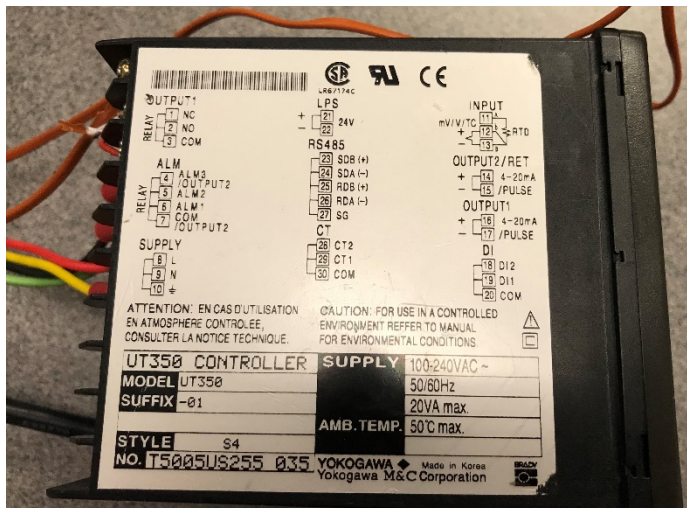
Figure 7.11: Yokogawa UT-350 Controller Wiring Backplane and Labels.
