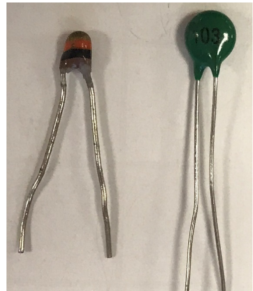
Figure 4.7: Two varieties of 10 kΩ NTC Thermistors ( Link to the left one ).
