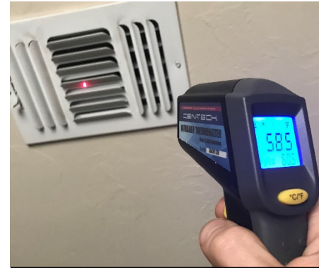
Figure 4.2: Measuring the temperature of the air coming out of a vent with an infrared thermometer (or pyrometer).
