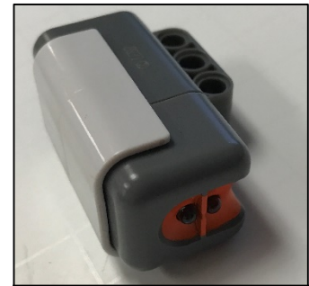
Figure 4.24: Photo of the NXT reflection sensor. The LED and phototransistor look like glass beads.
