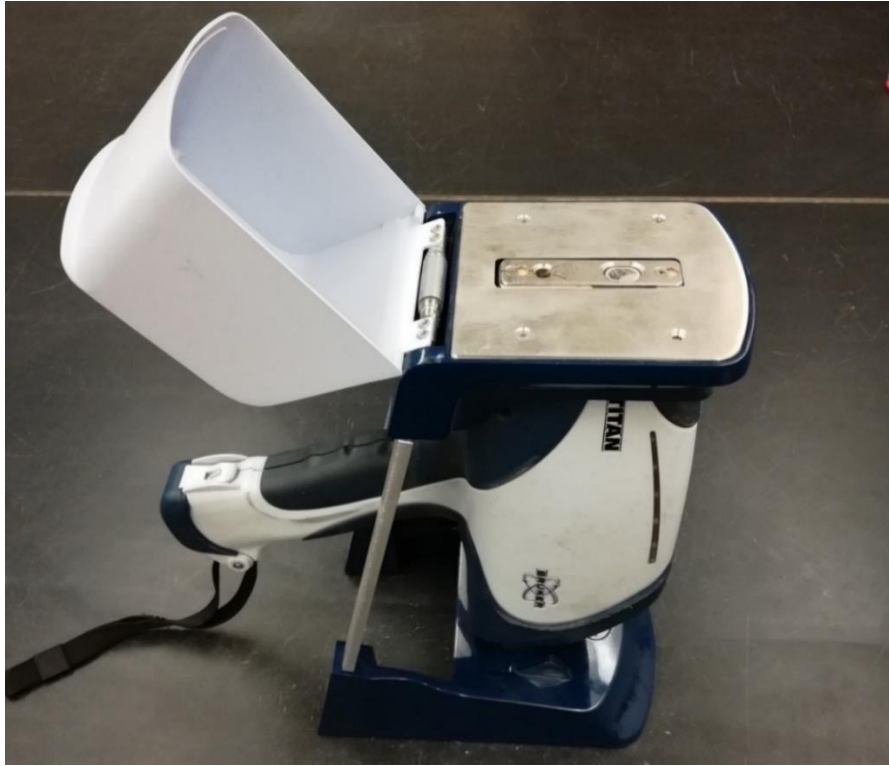
Figure 8: S1 TITAN from Bruker mounted in the testing stand
