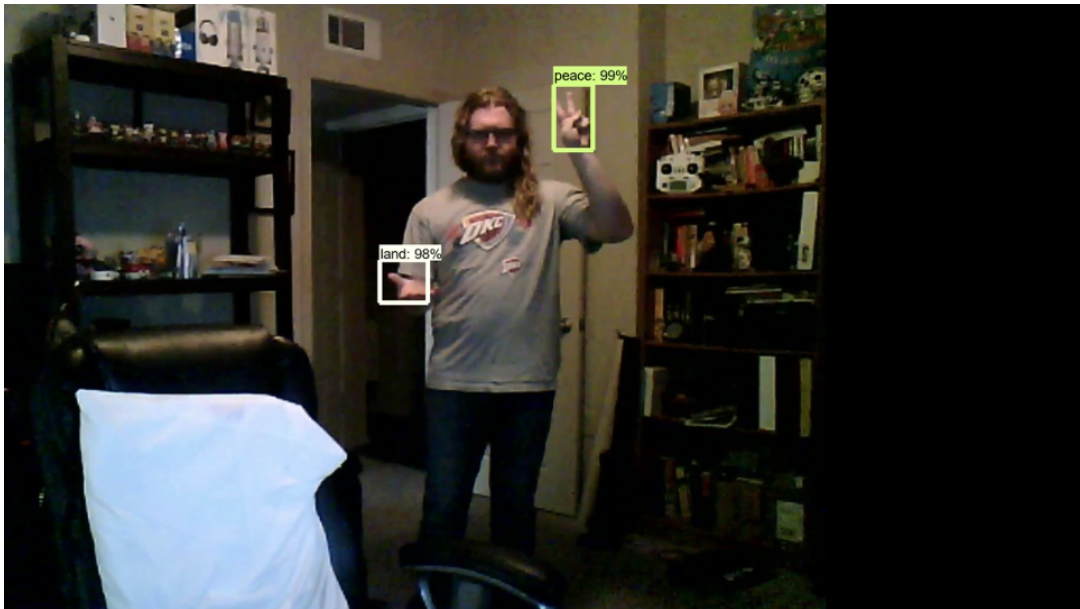
Figure 2.26: A frame with two classified gestures. The protocol would interpret this frame as a terminating frame since “land” is a termination action and is always be considered first for safety rather than the higher percentage “peace” gesture.
