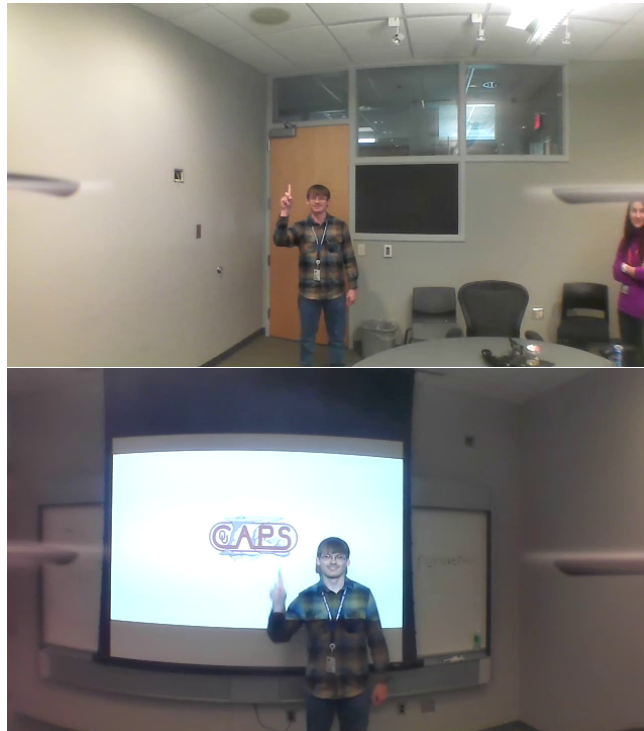
Figure 3.3: Two “up” gestures: one with no harsh light and a clear background, and one with a brightly lit projector screen.
