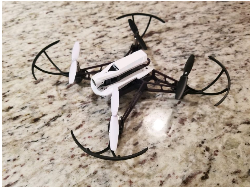
Figure 2.22: The Parrot Mambo Fly drone used in this thesis. Here, it has the added camera attachment.
