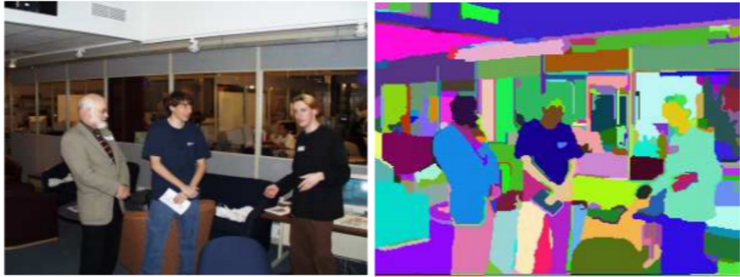
Figure 2.9: Complete segmentation on an indoor scene. Each color on the output image (right) identifies a different component such as a face, a shirt, a nametag, or a book from the input image (left). Image from Felzenszwalb and Huttenlocher 2004.
