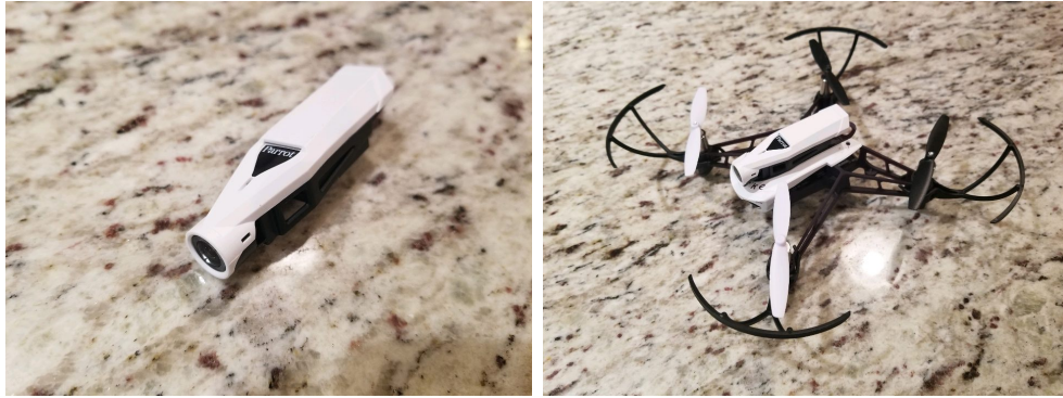
Figure 3.1: The mini-drone camera attachment, both separated and installed on the mini-drone.
