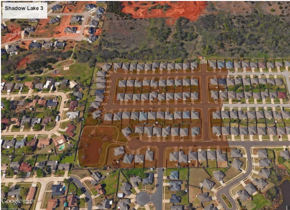
Figure 9: The drainage area of the Shadow Lake #3 drainage area and its corresponding retention pond
