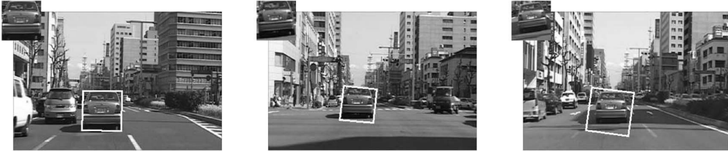
Figure 2.6: Background leakage example [20]©IEEE 2004
