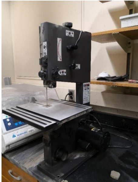
Figure 1 Band saw (it has no teeth) used to cut shale into chunks
