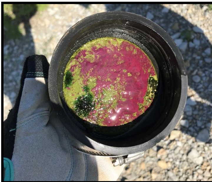
Figure 5.4. Purple sulfide oxidizing bacteria seen in a cap on the Vertical Flow Bioreactor (VFBR) effluent pipes
