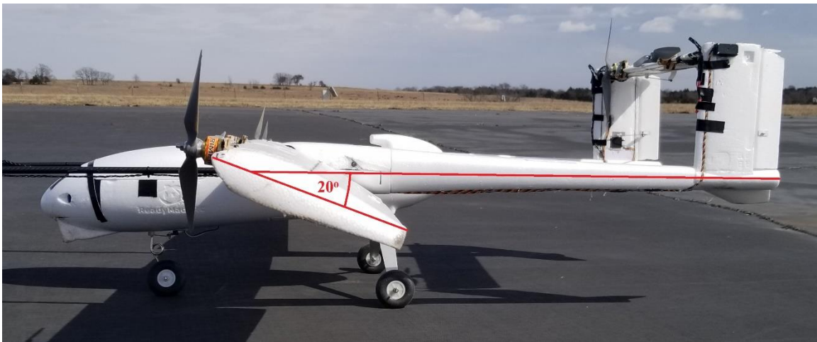
Figure 48: Wing rotated 20 degrees for STOL testing
