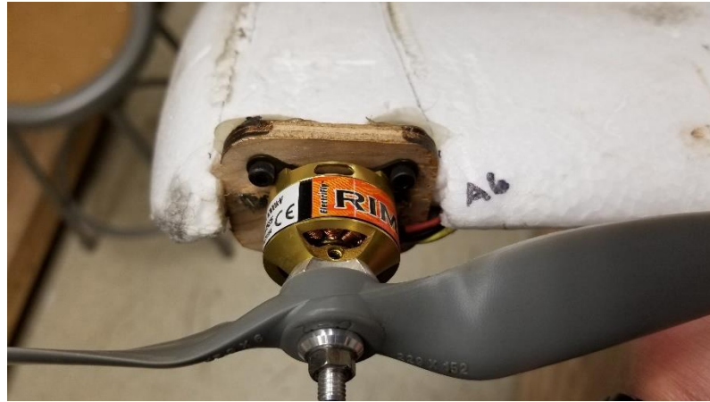
Figure 35: Plywood motor mount mounted on right wingtip. The mount was hot glued and pegged.
