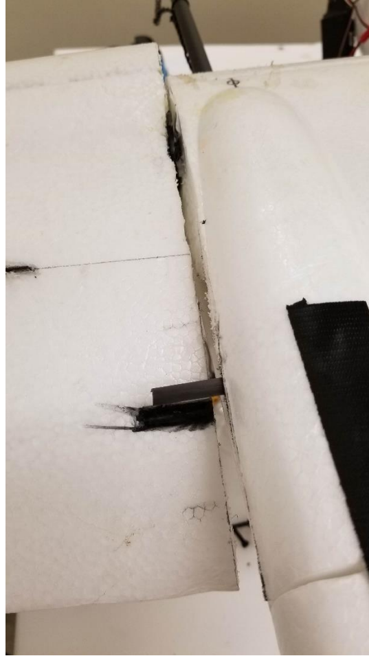
Figure 43: Wing rotation stop rod right before it locks into place. In this image, the main wing (to the left) has about a 20 degree rotation from horizontal
