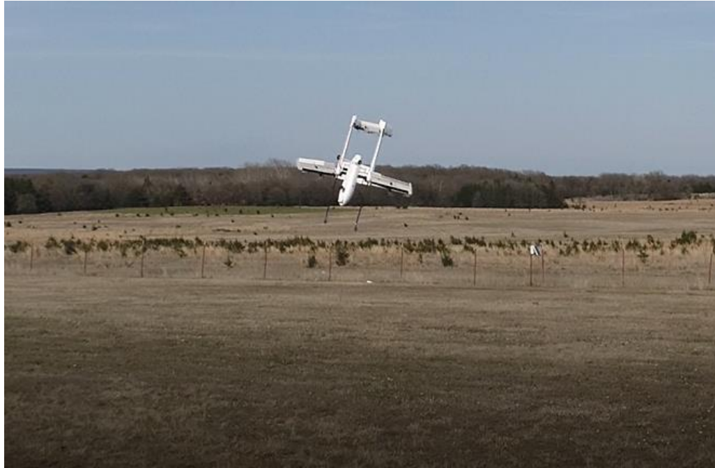
Figure 71: Image of aircraft pitched down 80 degrees as seen at point “d” in Figure 70, above.
