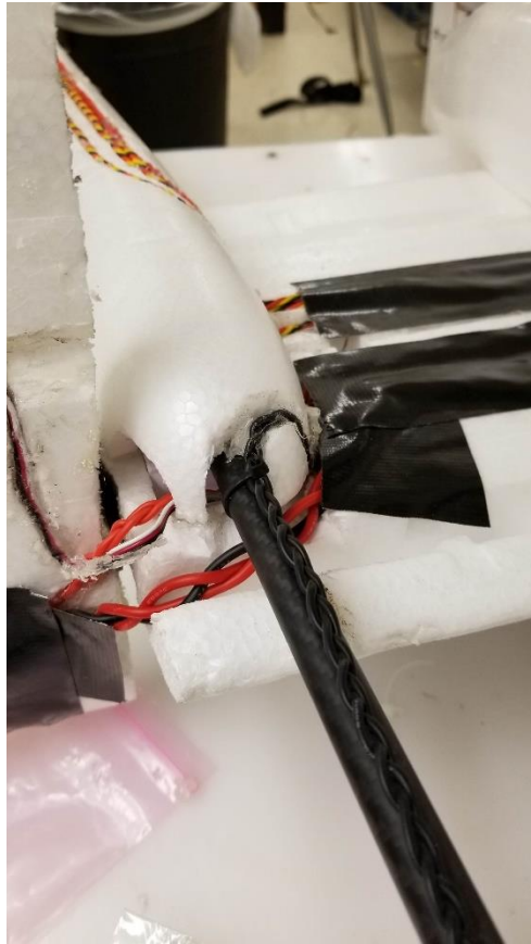
Figure 37: Boom extensions for placing the boom motors forward of the center of gravity.
