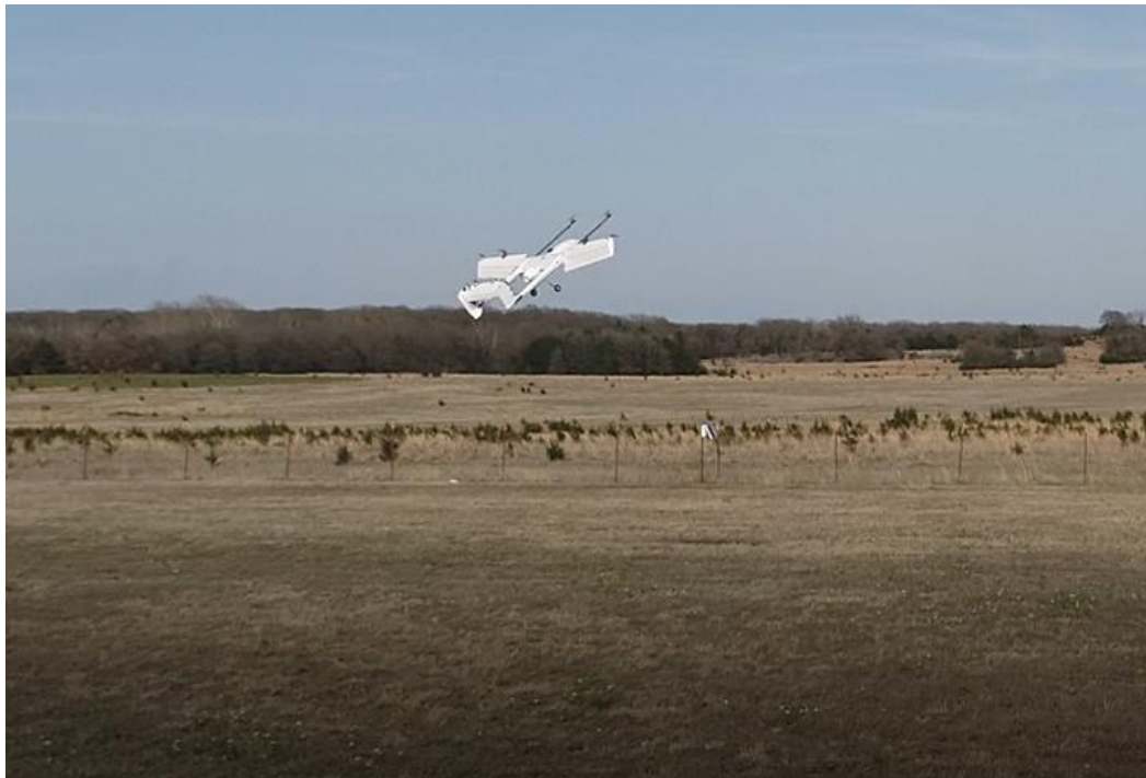
Figure 70: Image of aircraft pitched up 61 degrees as seen at point "c" in Figure 70, above
