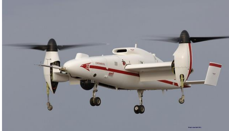
Figure 4: Bell Eagle Eye in the hover/VTOL phase of flight. Picture from Drew [9].
