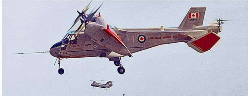
Figure 9: Canadair CL-84 in the transitional flight phase. Picture from Royal Aviation Museum of Western Canada [28].
