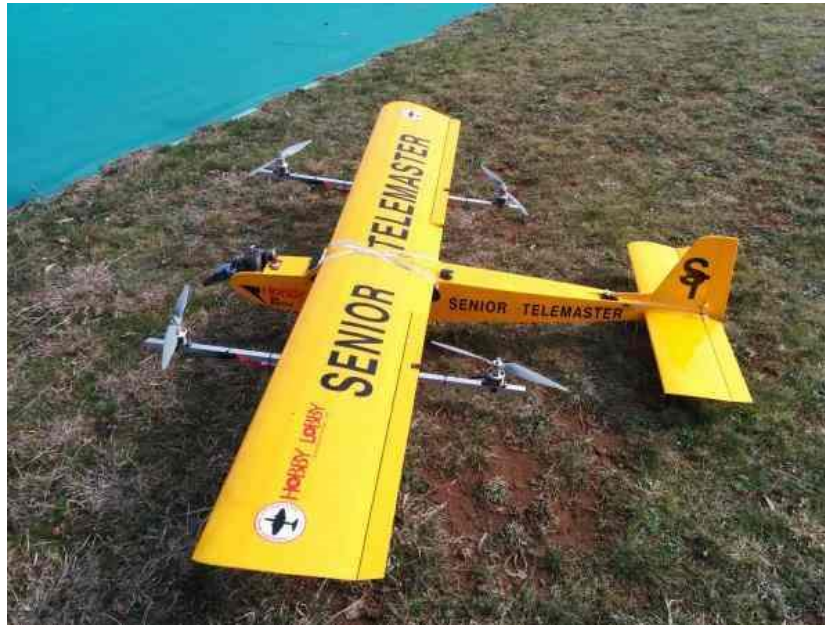
Figure 50: A typical quad-plane setup. The electric motors spin up for vertical take-off, and slowly turn off as the forward flight propulsion system slowly turns on. This process happens in reverse for landing. Image from Advanced Precision Composites [38].
