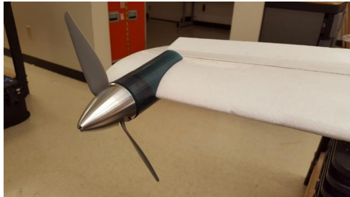
Figure 28: 3D printed motor pod with motor, propeller, and spinner mounted to RMRC Anaconda wing.
