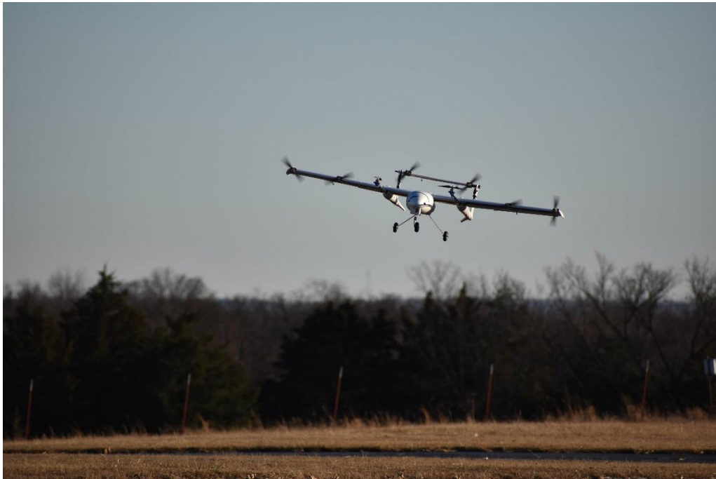
Figure 46: ElectraWing phase II flight test I. in this picture, the aircraft was landing in the CTOL configuration. Image by Antonio Valencia.
