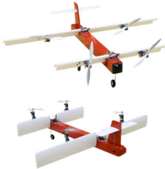
Figure 15: The QUX-02 airframe in transitional (top) and vertical (bottom) flight configurations. Picture from Dornheim [15].
