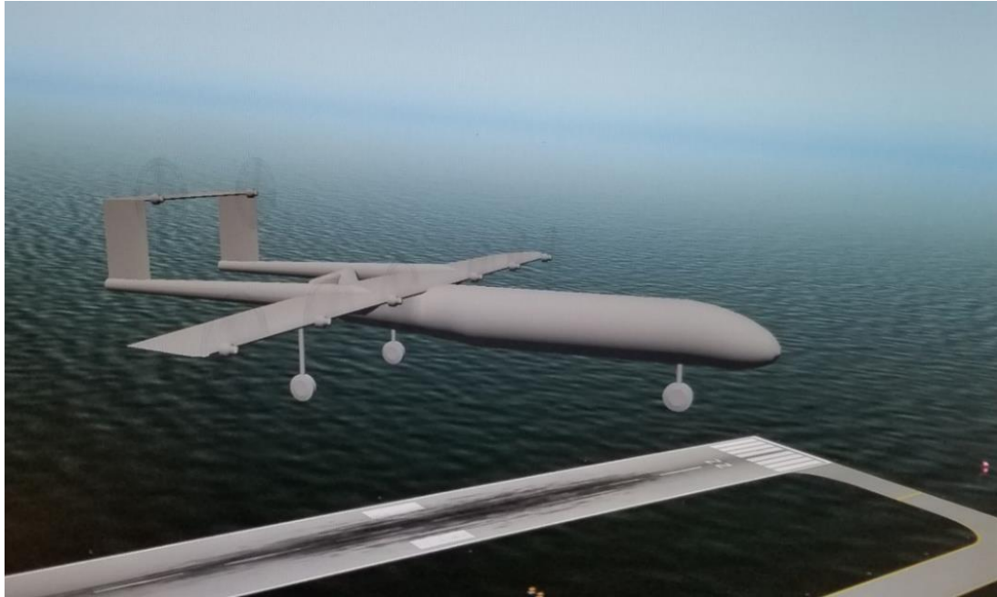
Figure 36: XPlane 10 simulation of the extended nose concept of ElectraWing.
