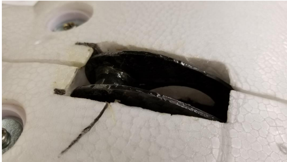
Figure 41: Control horns attached to the wing tube after the assembly was complete. As pictured, the wings are in the horizontal configuration. A section in the middle of the wings had to be cut away as to allow room for the control horns.
