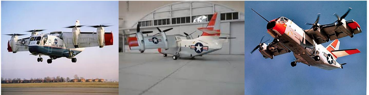
Figure 11: LTV XC-142A in VTOL configuration (left). The aircraft has a tilting wing to transition between vertical and forward flight. In the middle image, it can be seen that it has a rotor on the tail that rotates in the horizontal plane to ensure stability when in the vertical flight configuration. This rotor stops rotating when in forward flight. On the right, the aircraft can be seen in the forward flight configuration. Pictures from Ozdemir [4] and globalsecurity.org.
