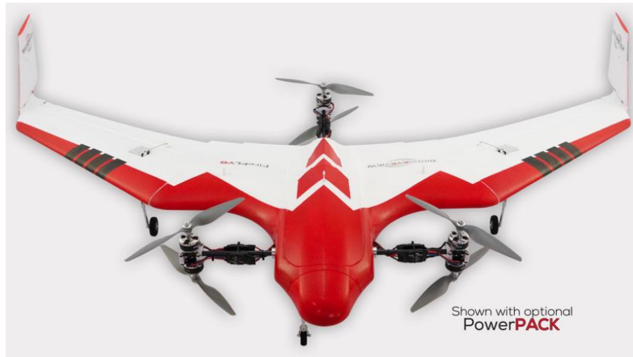
Figure 51: BirdsEyeView FireFly platform. When this aircraft takes off vertically, all three sets of motors are vertical facing to provide lift, as the aircraft transitions, the front two sets of motors rotate to a horizontal configuration while the rear motors to a horizontal configuration while the rear motors turn off. The reverse happens for vertical landing. Image from ArduPilot.
