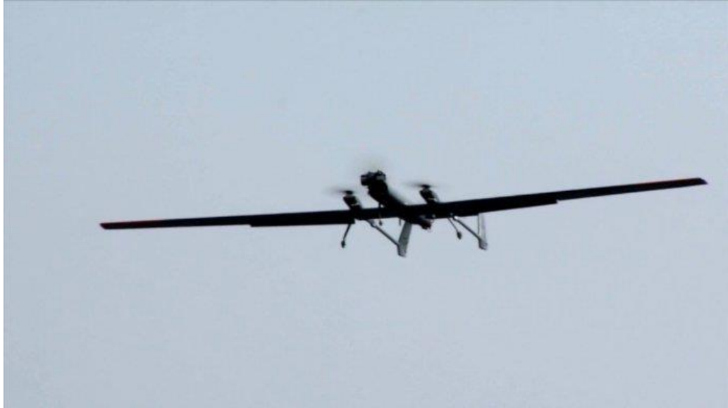
Figure 6: The Israel Aerospace Industries Panther-FE proof of concept in vertical flight. Image from Austin [8].
