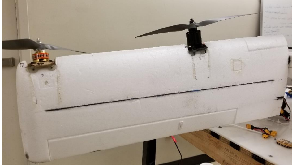
Figure 56: Larger motor on inboard of wing with original RimFire motor on wingtip
