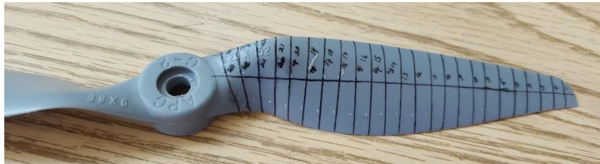
Figure 29: APC 9X6E divided into 24 segments for XROTOR analysis.
