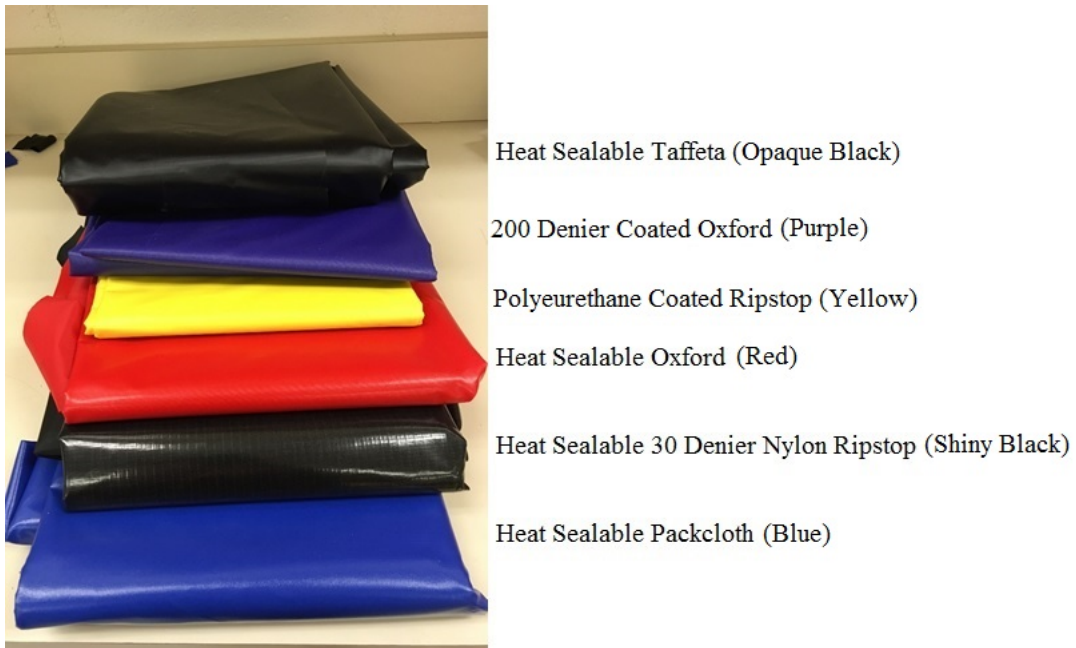
Figure 22: Six fabrics tested for heat seal ability
