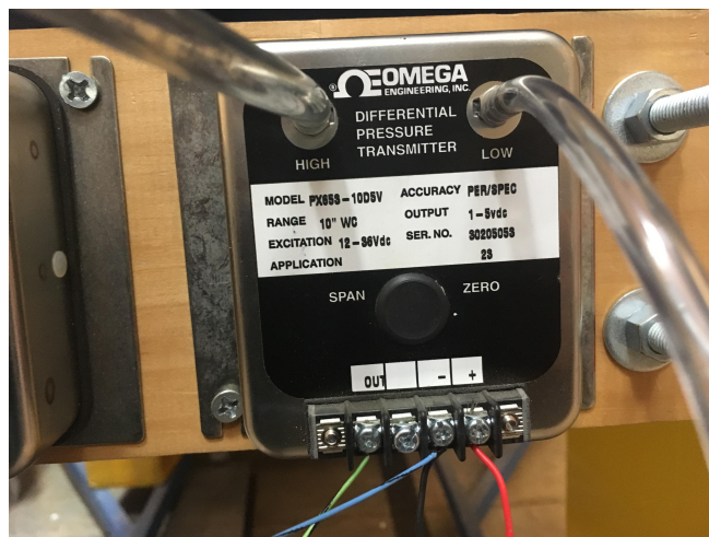
Figure 51: Omega 10inch pressure transducer
