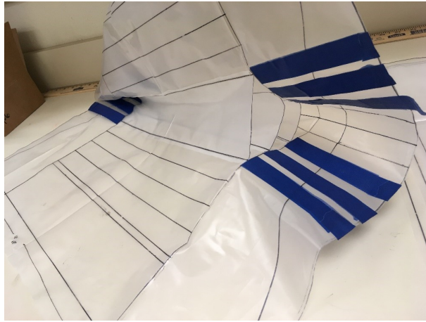
Figure 42: Initial heat sealed baffles
