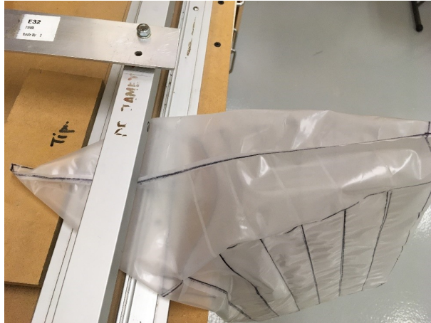
Figure 45: Heat sealing corners for proper shape
