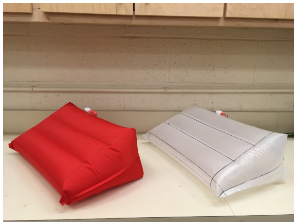
Figure 33: Inflated two-baffle boat-tail, HS Oxford and HS plastic sheeting
