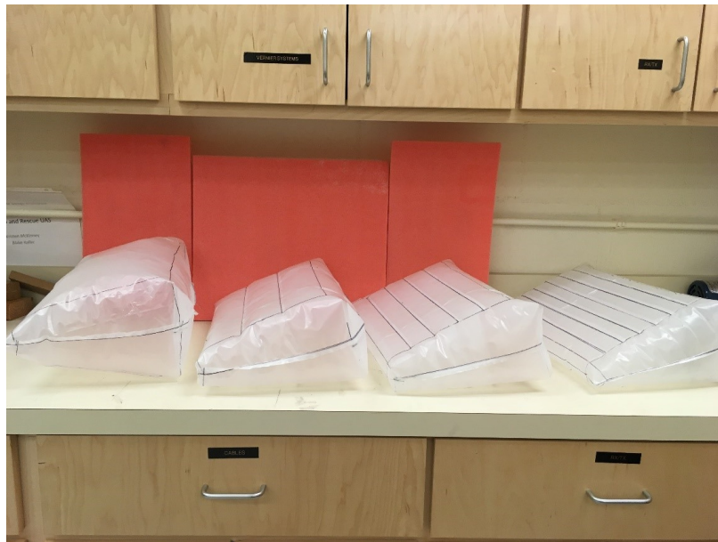
Figure 48: Comparison of shape for zero, two, four, and six-baffled boat-tails
