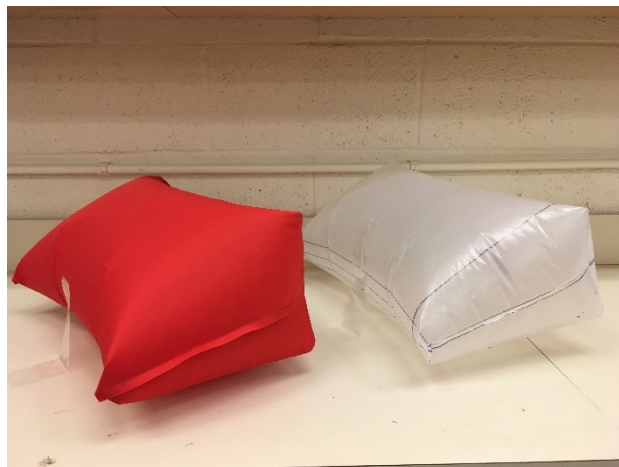
Figure 31: Inflated zero-baffle boat-tail, HS Oxford and HS plastic sheeting
