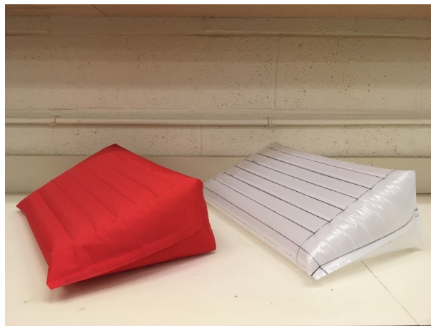
Figure 36: Inflated six-baffle boat-tail, HS Oxford and HS plastic sheeting
