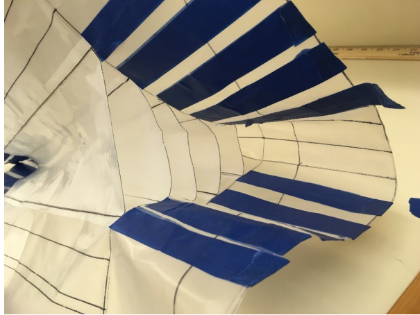
Figure 43: Heat sealed baffles
