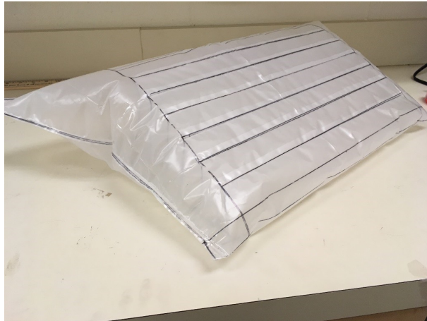
Figure 44: Edges heat sealed, partially inflated
