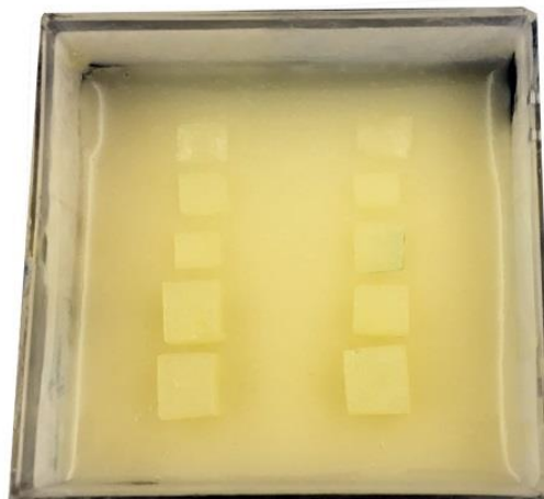
Figure 5-1: 70G-30A breast phantom embedded with gelatin blocks
