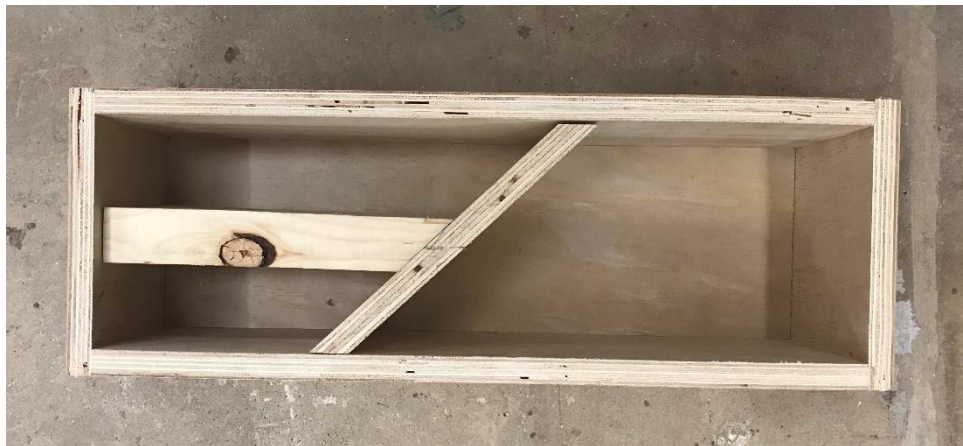
Figure 21: 45 degree exposed aggregate insert in MOR specimen form
