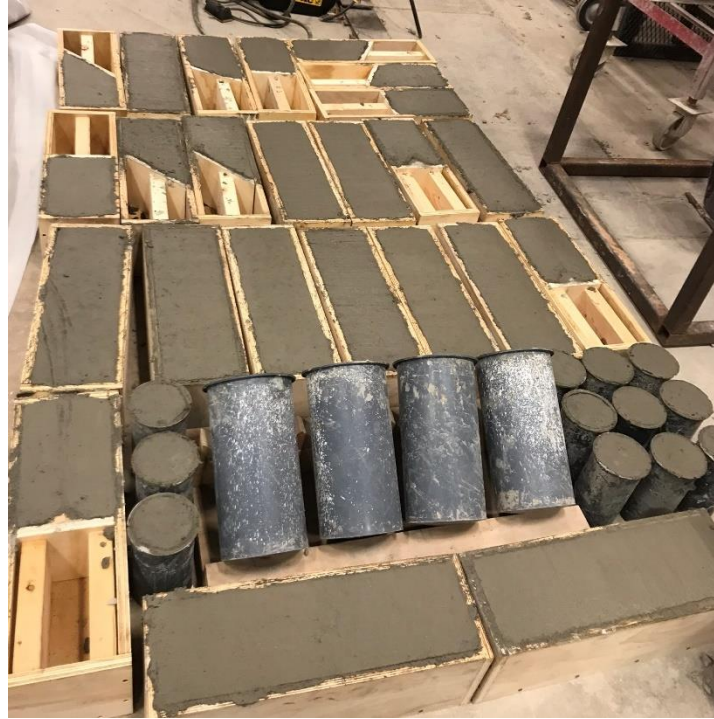
Figure 19: Composite MOR specimens after casting of NSC
