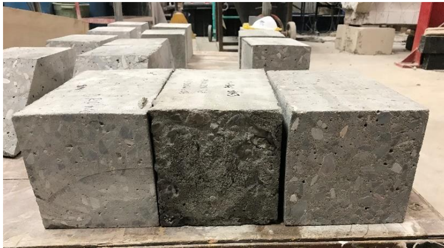
Figure 22: Wire brushed, exposed aggregate and sand blasted surface preparations (left to right)
