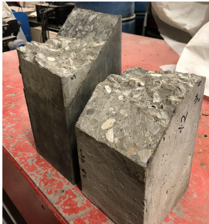
Figure 37: Composite MOR base concrete failure (8-SB-45)
