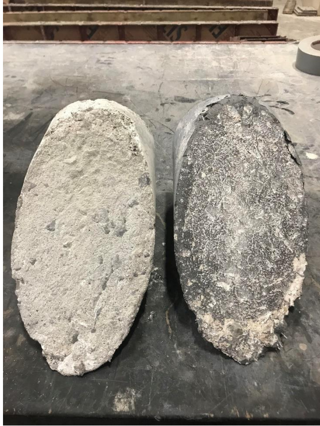
Figure 29: Slant shear specimen post failure
