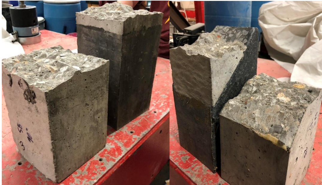
Figure 34: Base concrete failures (7-SB-90/3-WB-45)
