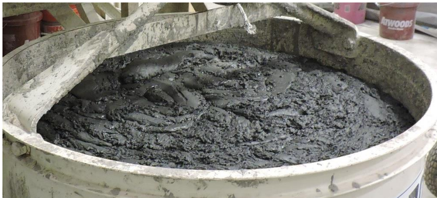
Figure 24: J3 UHPC alternative after mixing
