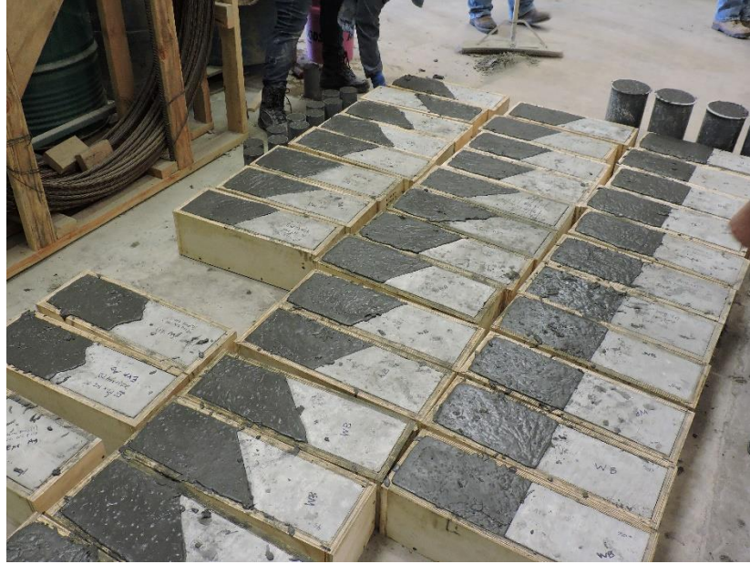
Figure 25: Composite specimens after casting
