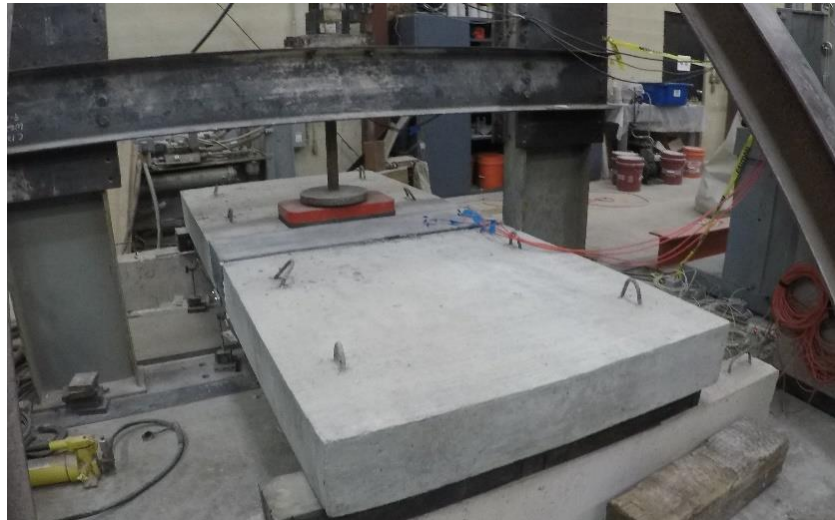
Figure 18: Test setup for slabs
