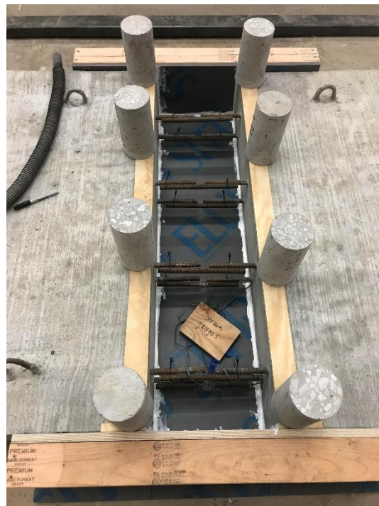
Figure 12: Positioned NSC panels
