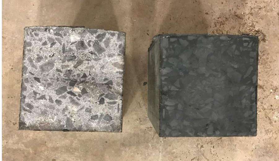
Figure 27: Composite MOR that failed during demolding
