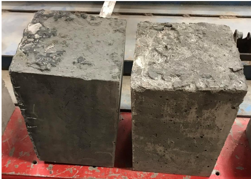
Figure 32: Interface failure (9-EA-90)
