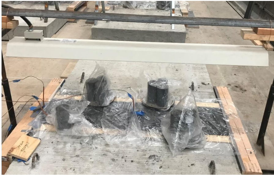
Figure 67: Slab joint during heat curing
