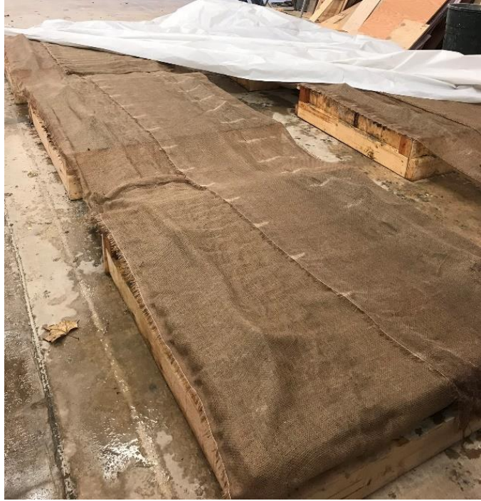
Figure 11: Panels curing under wet burlap
