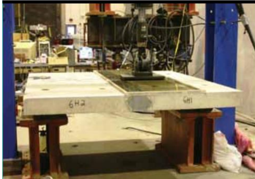
Figure 5: UHPC longitudinal connection cyclic test setup
