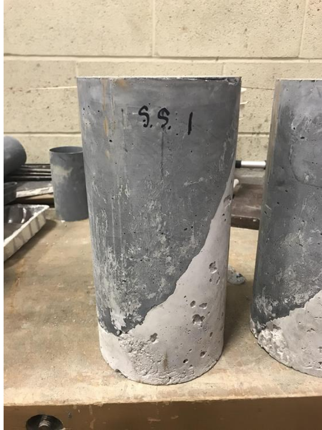
Figure 28: Composite slant shear specimen
