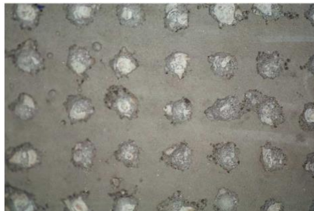
Figure 3: Partially Chipped Surface Preparation (Julio et al. 2004)
