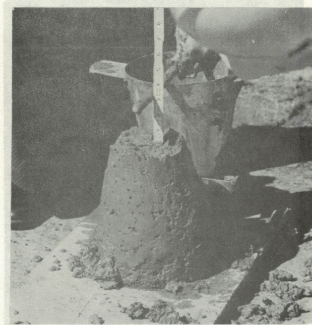
Figure 21: Inspector measures 3 inches of slump.
