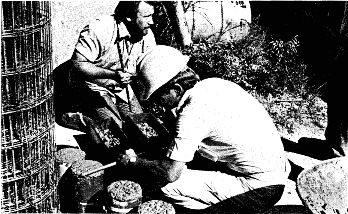
Photograph 5: Cylinders and beams were made from a trial mix of the wax bead concrete.
