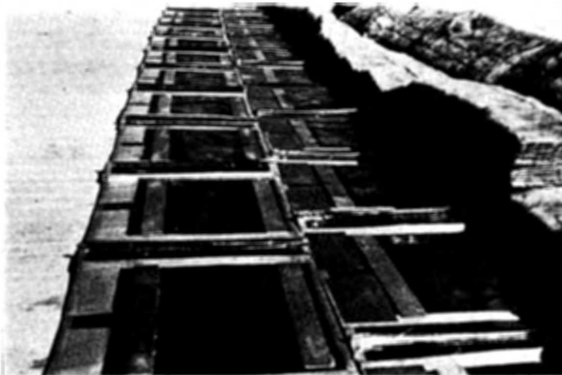
Photograph 18: A partial heat zone (no insulation) is set up around the perimeter of each heat run.
