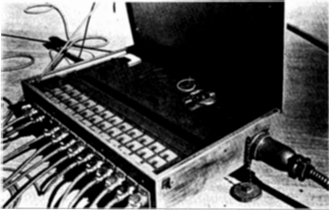
Photographs 15 & 16: Control console. Flashing red light would come on automatically if any of the circuits broke.
