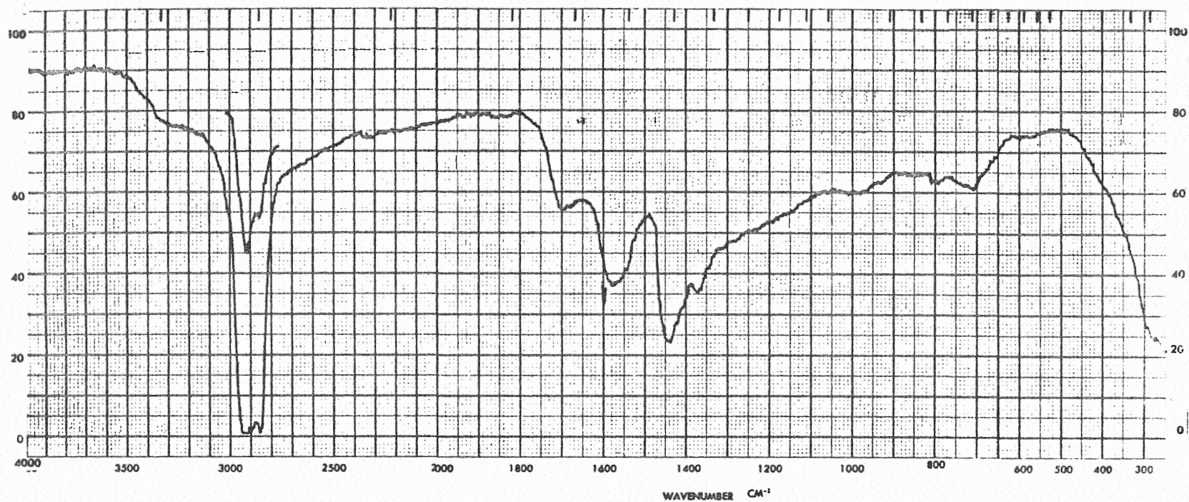
FIG.12 : Chem crete. This product was developed by the Chem-crete Corporation of Menlo Park, California. Chem-crete chemistry involves the addition of a small amount of common metal to promote oxidation and polymerization. This is observed by the presence of absorption at 1700 \text{ cm}^{-1} for C=O stretch.
