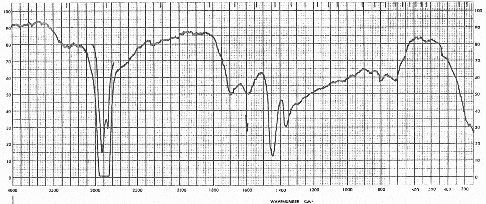
Figure 14c: Beaver County Road Core Asphalt Resins Fraction 401-03
