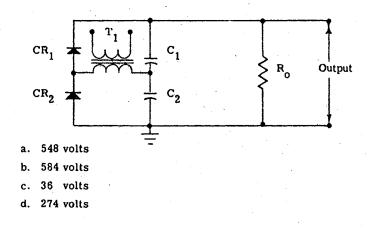
78. Does the presence of the capacitor-input filter between the half-wave rectifier and the load resistance in the circuit below have any effect on the peak inverse voltage applied across the diode?
