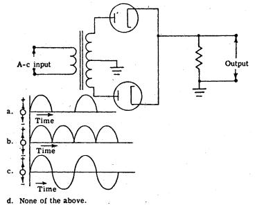
76. Which of the wave shapes below represents the output voltage of this circuit?
