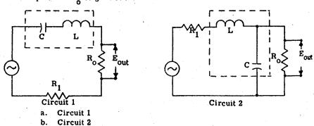
c. The voltage drop across  $R_0$  is the same in both circuits.
