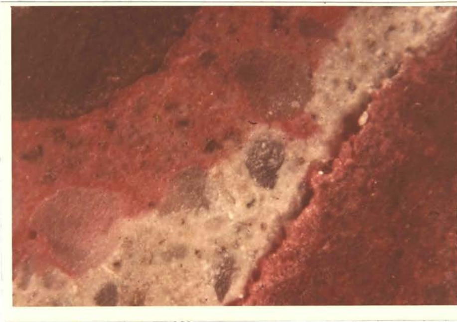
Figure 12. Aggregate Bond Crack on Core Sample Similar to Samples A1, A2, A3. Damage was Done Eight Years Prior to Photograph. Magnification is 51x
