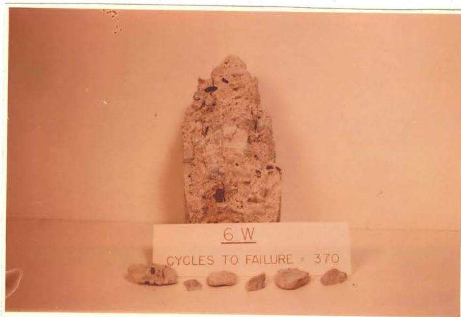
Figure 15. Ultimate Failure of Core Sample A3 Indicating a Bond Failure Around the Aggregates. Typical of Damaged Specimens
