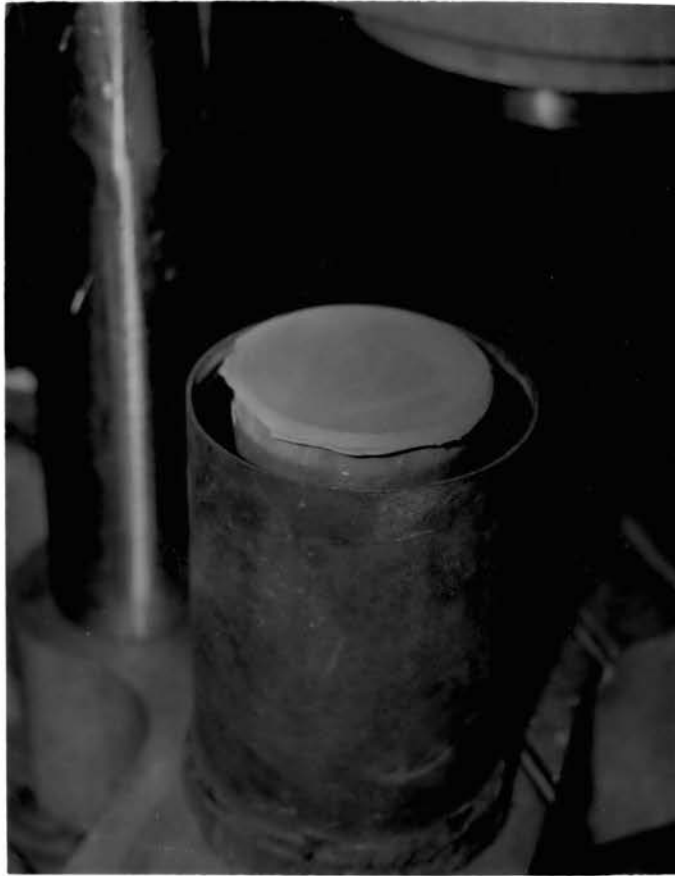
Figure 3. Special Apparatus Used to Maintain Complete Saturation During Slow Cycle Fatigue Testing
