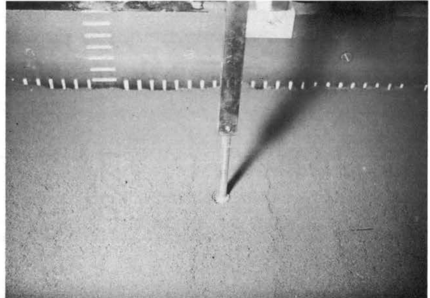
Figure 13. One Inch Diameter Bearing Plate on the Soil Surface and as it is Forced into the Soil
