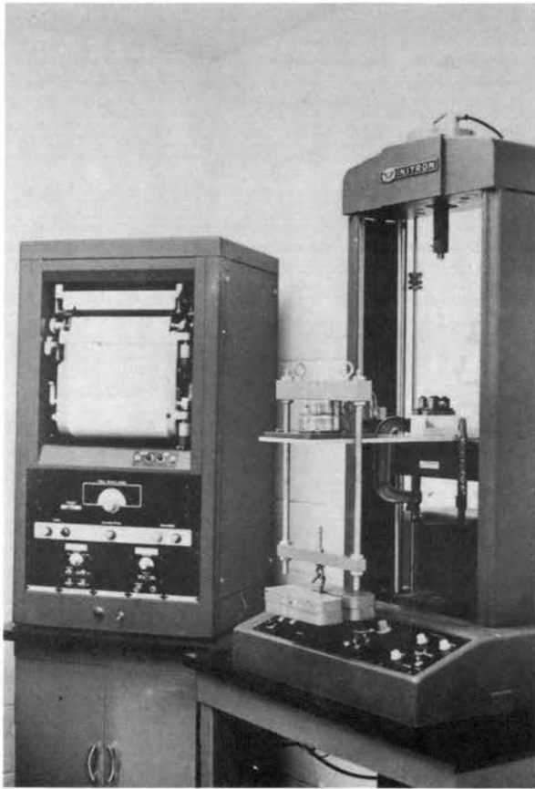
Figure 10. Instron Universal Testing Machine with a Direct Soil Shear Testing Apparatus
