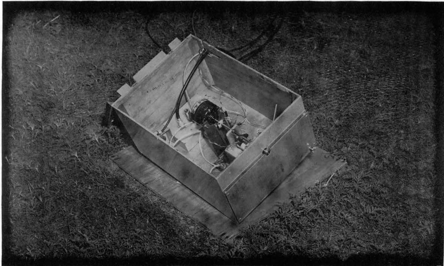
Figure 6.6. Exterior Portion of the Electric Fluxmeter
