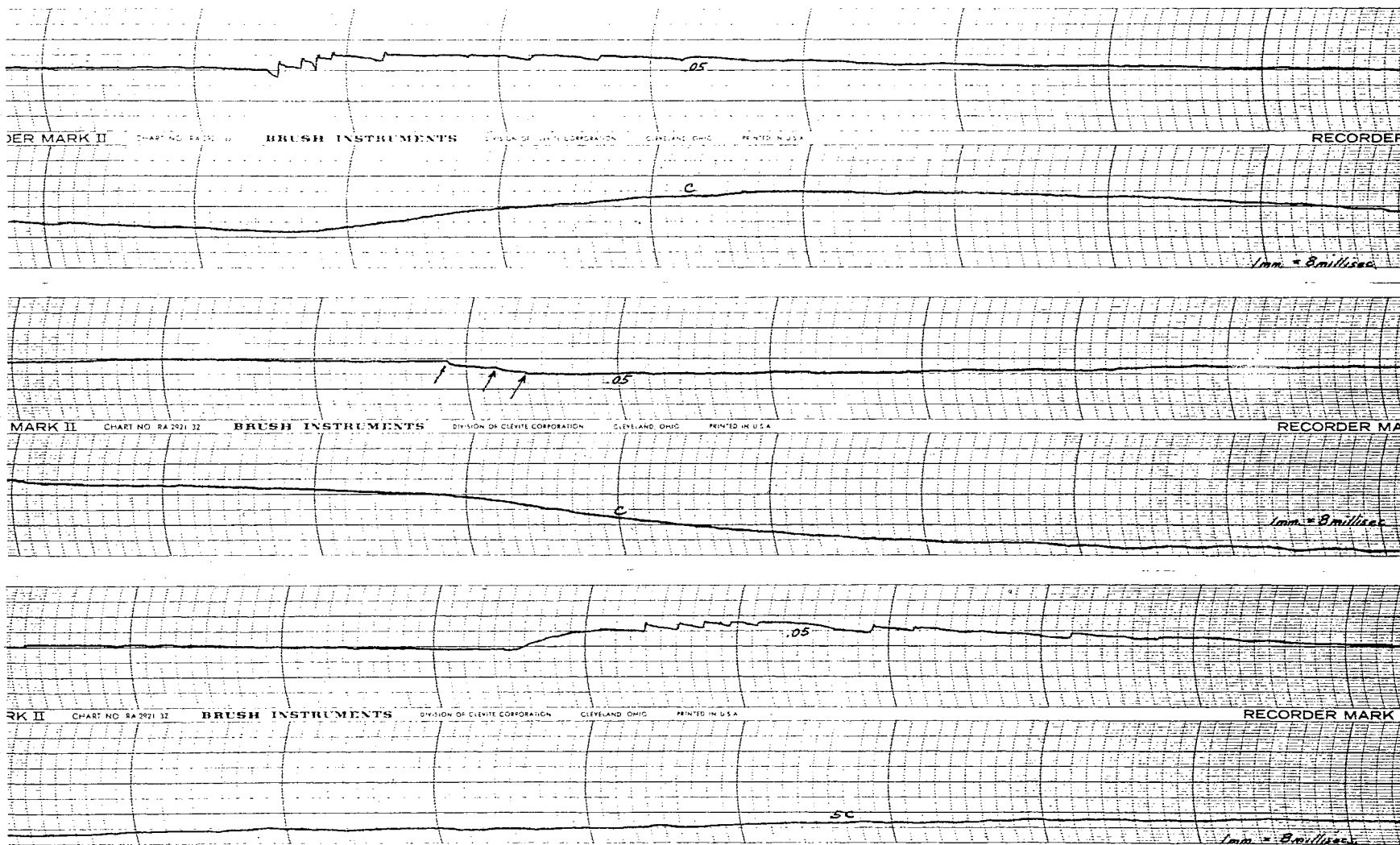
Figure 7.16. [Top to Bottom] Multiple strokes bringing about field reversal. Three intra-cloud strokes and their effect on the field; series of cloud-to-ground strokes with very high mean field. [8 kilovolts/meter]
