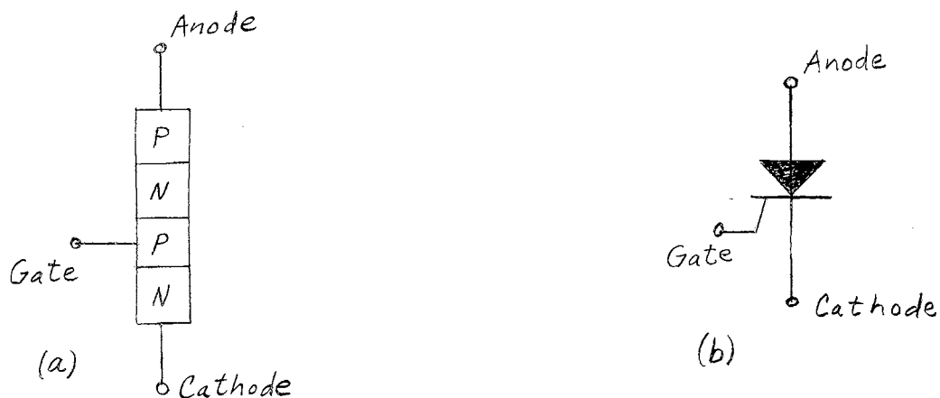
Figure 1. (a) Crystalline Structure of a Silicon Controlled Rectifier. (b) Symbol of a Silicon Controlled Rectifier.
