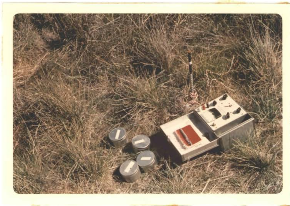
Figure 7. Measuring Soil Moisture and Temperature as Current Flow Through Coleman Soil Cells
