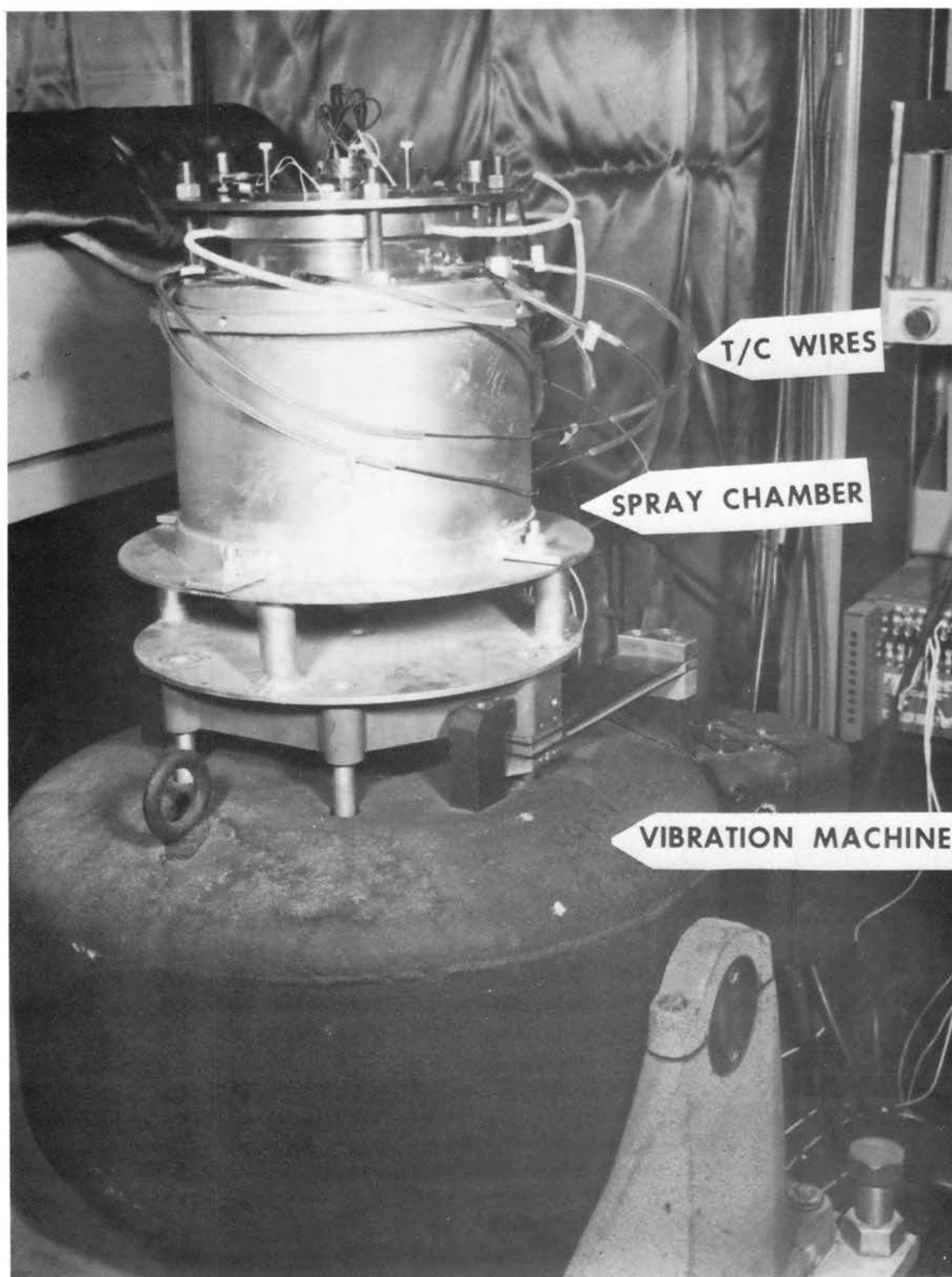
FIGURE 3- TEST APPARATUS ASSEMBLED
