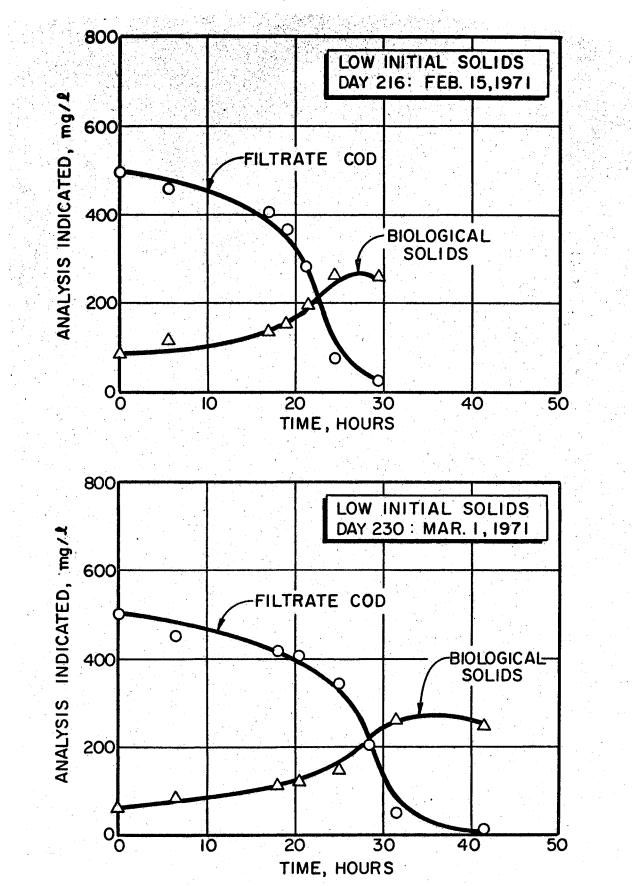
Figure 46. Response of the extended aeration activated sludge to a slug dose of glucose after 250 days of operation and after 272 days of operation.
