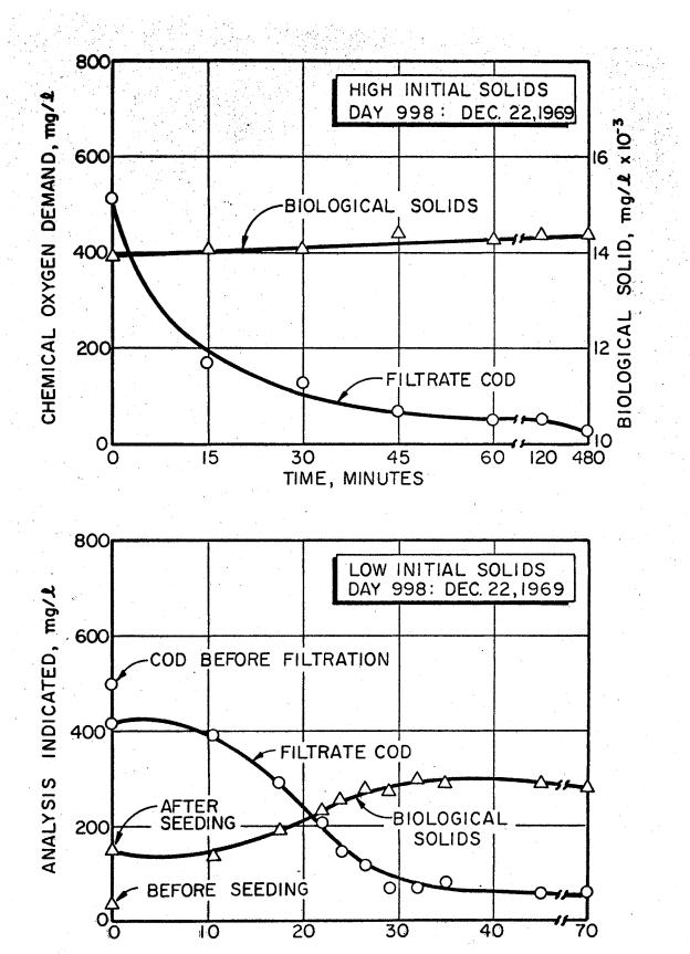
Figure 29. Metabolism of hydrolyzed extended aeration sludge using a low initial inoculum of cells taken from the extended aeration activated sludge pilot plant on day 1097 (March 31, 1970).
