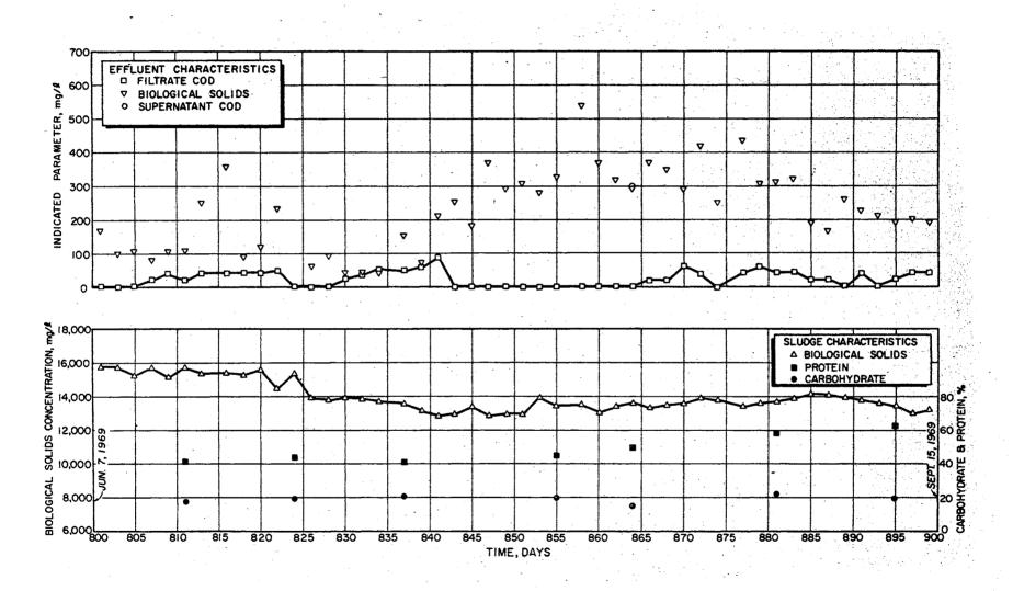
Figure-13: Performance-data-for continuous flow extended aeration pilot plant, September-15, 1969; to December-24, 1969.
