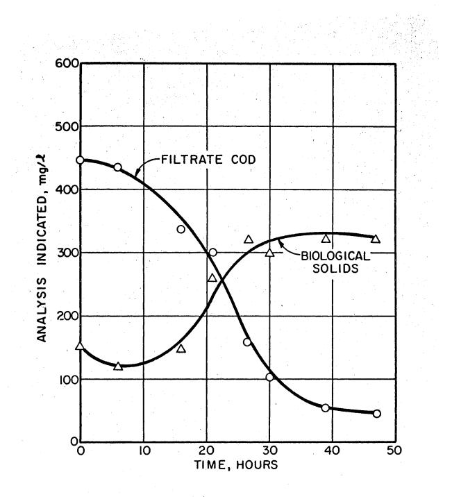
Figure 28. Metabolism of hydrolyzed biological sludge by extended aeration activated sludge at both low and high initial solids levels on day 998 (December 22, 1969).
