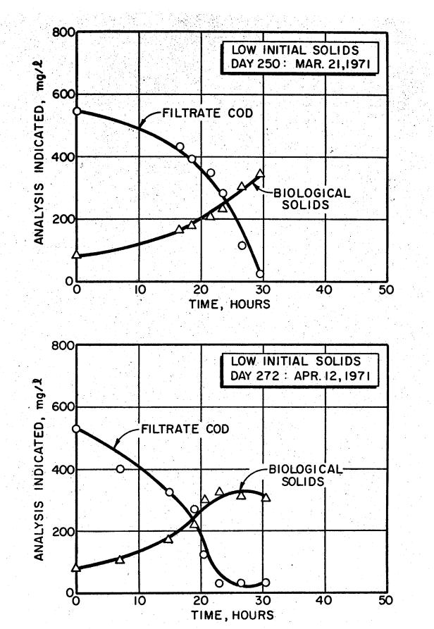
Figure 47. Response of the extended aeration activated sludge to a slug dose of glucose after 307 days of operation and after 308 days of operation.
