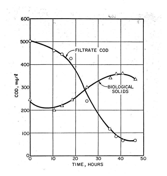
Figure 27. Metabolism of hydrolyzed biological sludge using a low initial inoculum of cells taken from the extended aeration activated sludge pilot plant on day 955 (November 9, 1969).
