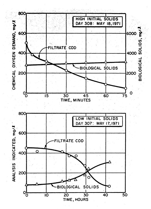
Figure 48. Response of the extended aeration activated sludge to a slug dose of glucose after 316 days of operation.
