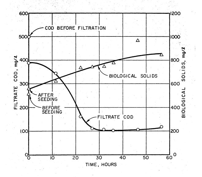
Figure 33. Metabolism of hydrolyzed biological sludge which had been previously flocculated using  $A1_2(S0_4)_3 \cdot 18$  H<sub>2</sub>0, 200 mg/1.
