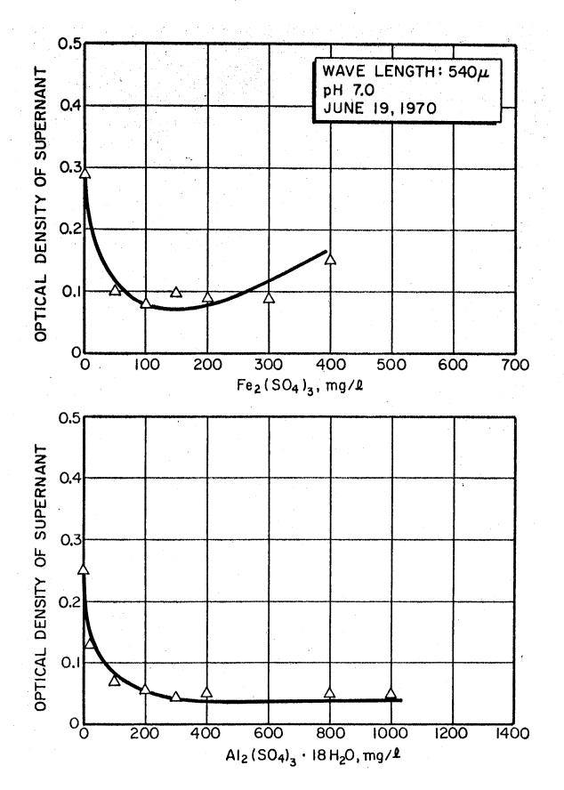
Figure 22. Effect of pH on the flocculation of biological solids retained in the effluent of the extended aeration pilot plant by the application of ferric sulfate and aluminum sulfate at the concentrations indicated.
