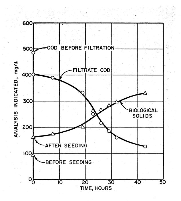
80 percent of the cell hydrolysate was soluble (i.e., passed through a 0.45 µ membrane filter). The hydrolysate was utilizable by a mature (extended aeration) activated sludge microbial population. The experiments were terminated after about 40 hours, and the residual COD was somewhat higher than when hydrolysate from younger cells was employed (compare residual COD in Figures 29 and 30 with those in Figures 25, 26, 27, and 28).
