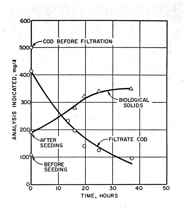
Figure 30. Metabolism of hydrolyzed extended aeration sludge using a low initial inoculum of cells taken from the extended aeration activated sludge pilot plant on day 1169 (June 11, 1970).
