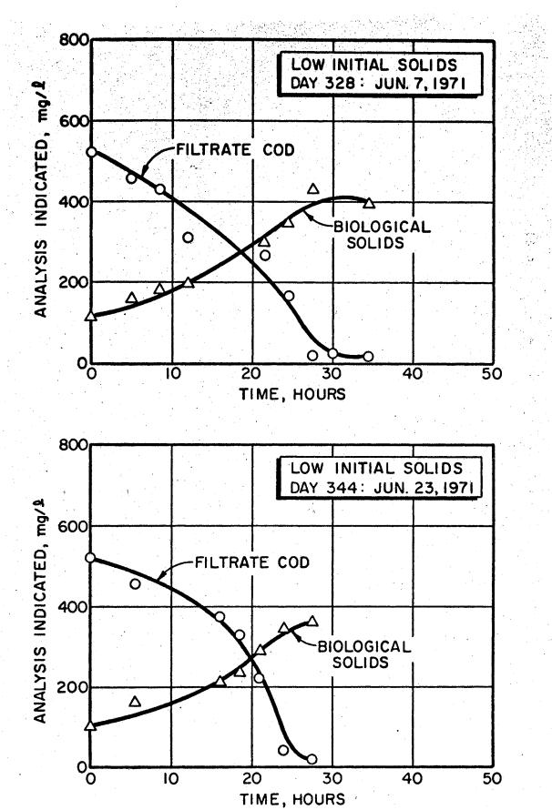
Figure 52. Response of the extended aeration activated sludge to a slug dose of sludge hydrolysate after 351 days of operation.
