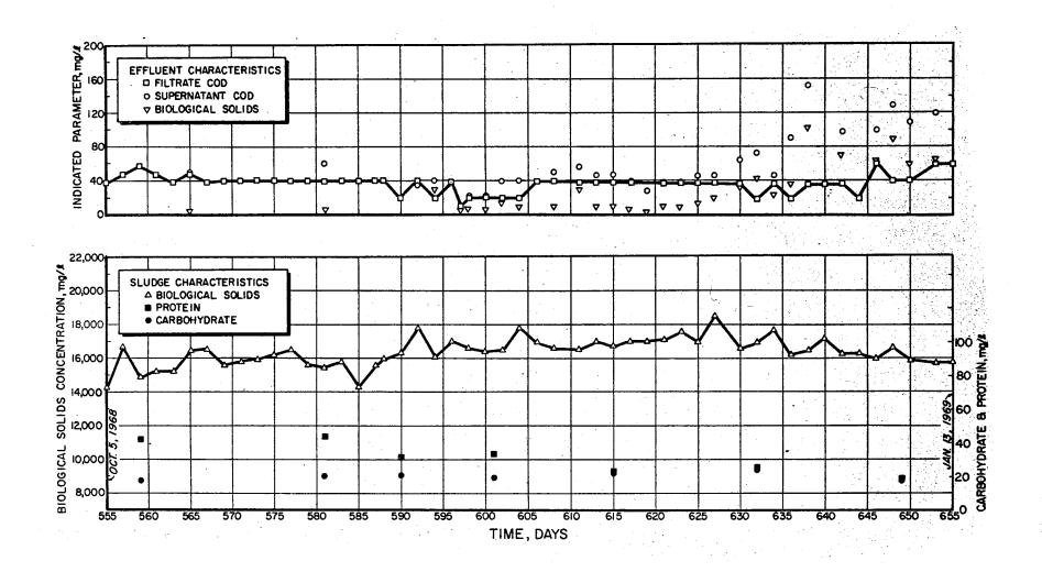
Figure 10. Performance data for continuous flow extended aeration pilot plant, November 19. 1968, to February 27. 1969.
