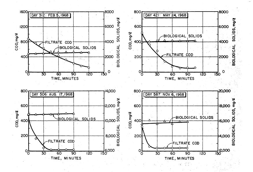
Figure 19. COD removal capability of extended aeration activated sludge on the day indicated.
