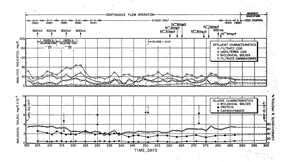
Figure 37. Operational characteristics of the extended aeration pilot plant with periodic withdrawal, hydrolysis and refeeding of portions of the activated sludge; days 300-388 (May 10, 1971, to August 6, 1971).
