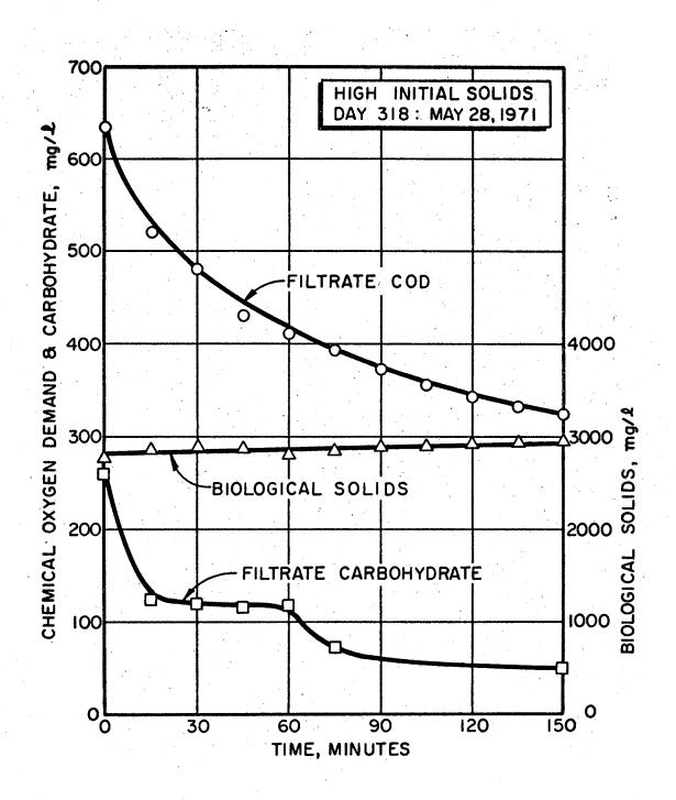
Figure 51. Response of the extended aeration activated sludge to a slug dose of glucose after 328 days of operation and after 344 days of operation.
