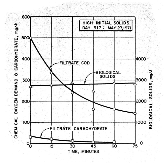
Figure 50. Response of the extended aeration activated sludge to a slug dose of sludge hydrolysate after 318 days of operation.
