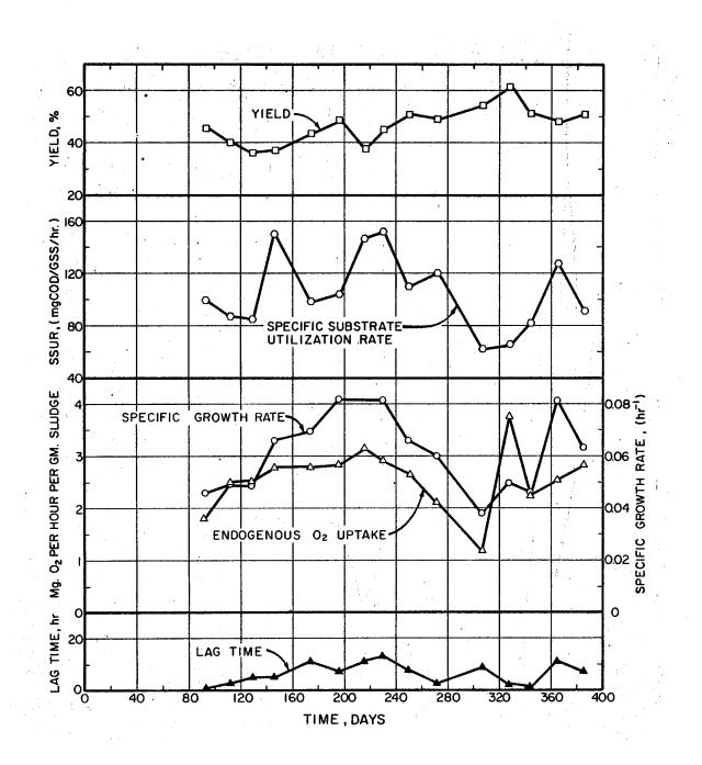
Figure 42. Response of the extended aeration activated sludge to a slug dose of glucose after 93 days of operation and after 112 days of operation.
