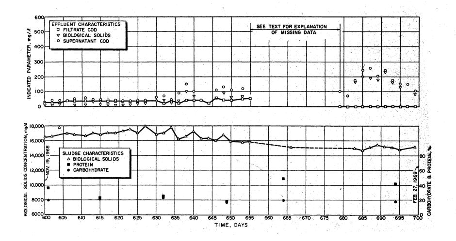
Figure 11. Performance data for continuous flow extended aeration pilot
