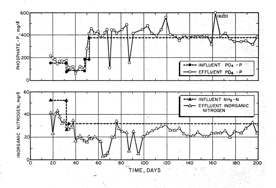
Figure 39.2 Comparison of phosphorus and nitrogen in the feed and in the feed and it is the feed and it is the effluent of the extended aeration pilot plant (January 30, 1971, ito July 27, 1971).
