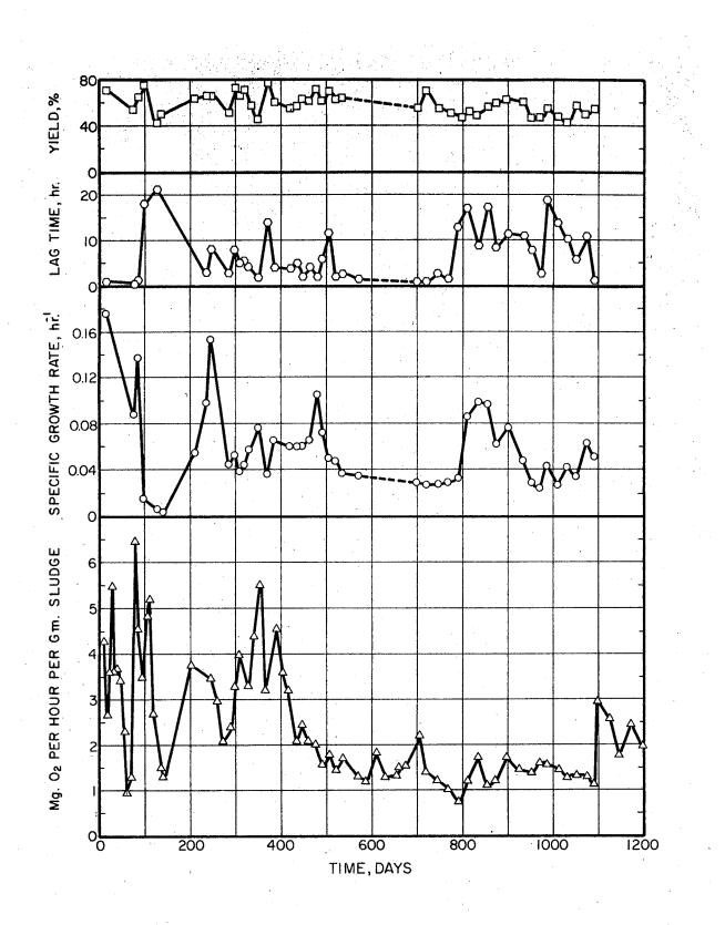
operation, the unit O2 uptake showed a sharp increase to 3 mg O2/hr/gm sludge. The rise corresponds to the time the unit was re-started (see Figures 14 and 15).
