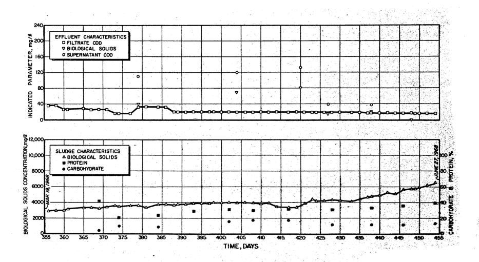
Figure 8. Performance data for continuous flow extended aeration pilot plant, June 27, 1968, to October 5, 1968.
