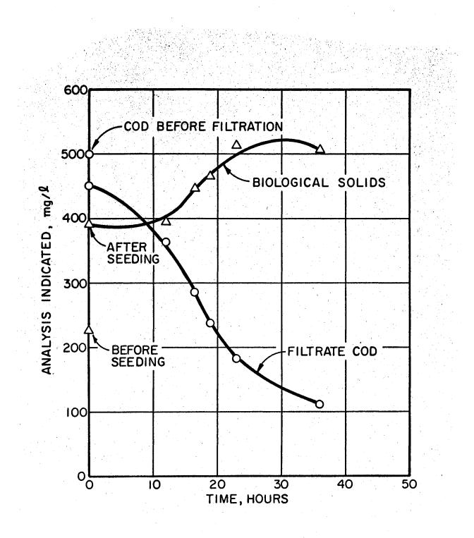
Figure 32. Metabolism of hydrolyzed biological sludge which had been previously flocculated using Al<sub>2</sub>(SO<sub>4</sub>)<sub>3</sub>·18 H<sub>2</sub>O, 200 mg/1.
