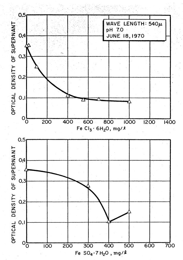
Figure 21. Effect of concentration of indicated coagulant on the flocculation of biological solids retained in the effluent of the extended aeration pilot plant.
