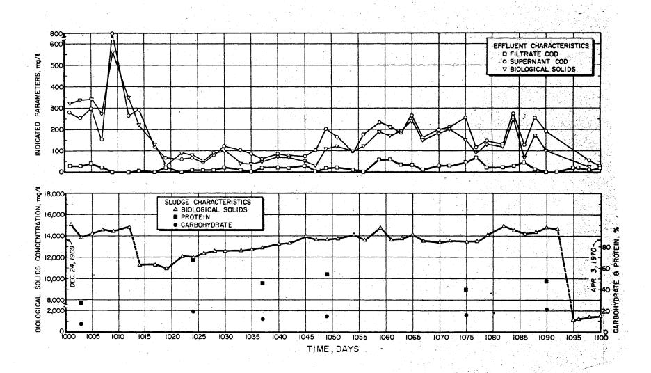
Figure 15. Performance data for continuous flow extended aeration pilot
