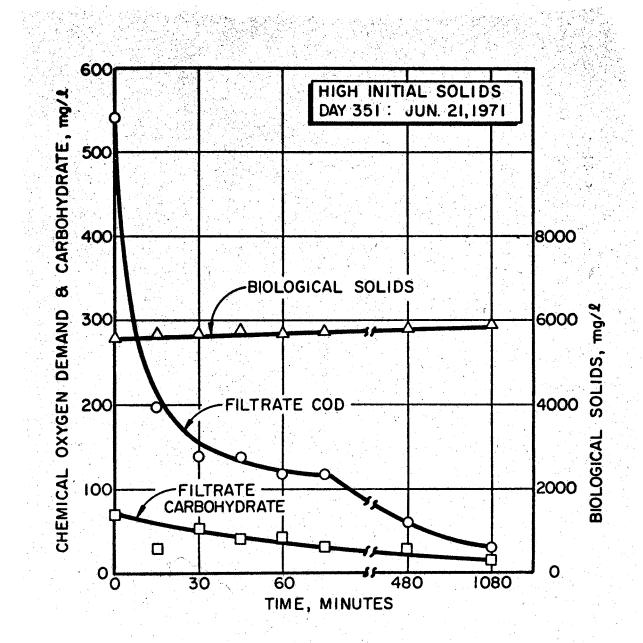
Figure 53. Response of the extended aeration activated sludge to a slug dose of glucose after 365 days of operation and after 386 days of operation.
