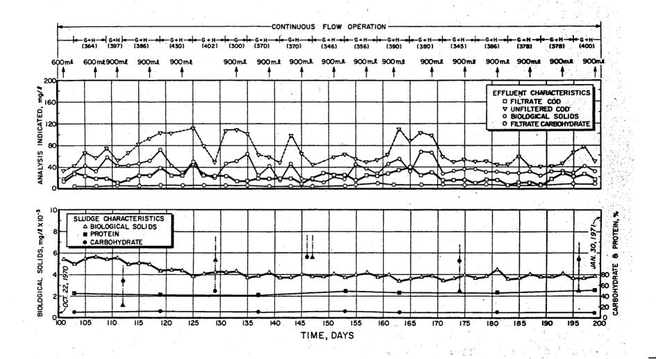
Figure 36: Operational characteristics of the extended aeration pilot plant with periodic withdrawal, hydrolysis and re-feeding of portions of the activated sludge; days 200-300 (January 30, 1971, to May 10, 1971).
