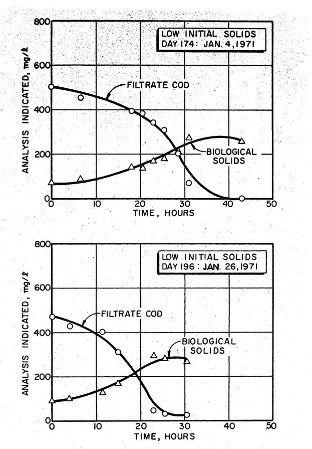
Figure 45. Response of the extended aeration activated sludge to a slug dose of glucose after 216 days of operation and after 230 days of operation.
