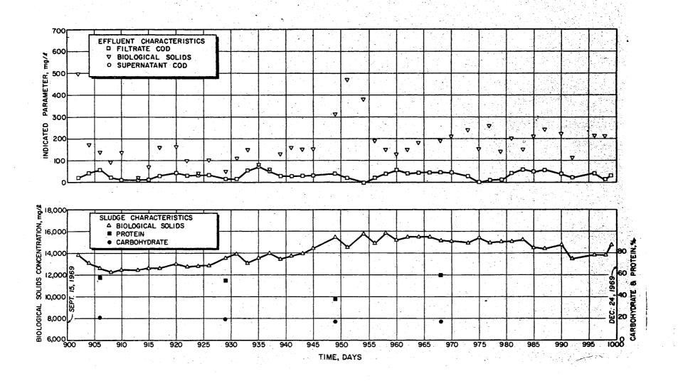
Figure 14. Performance data for continuous flow extended aeration pilot plant, December 24, 1969, to April 3, 1970.
