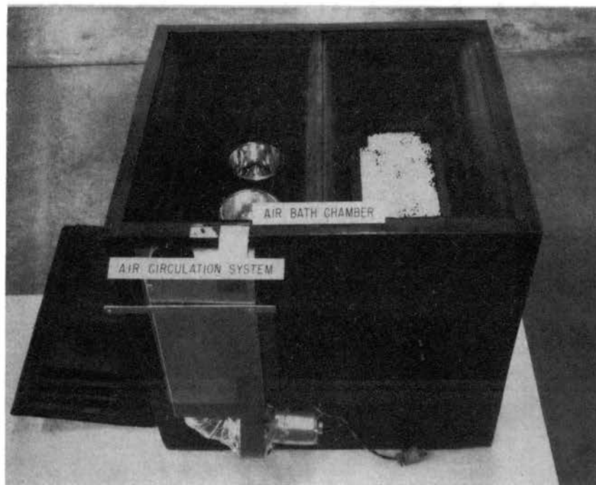
Figure 20. Air Bath Chamber and Air Circulation System
