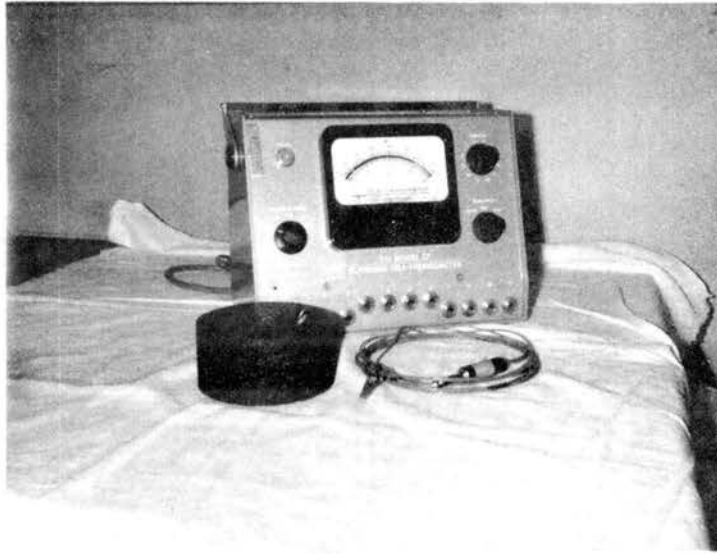
Figure 20. Temperature Monitoring Apparatus With Sample Specimen
