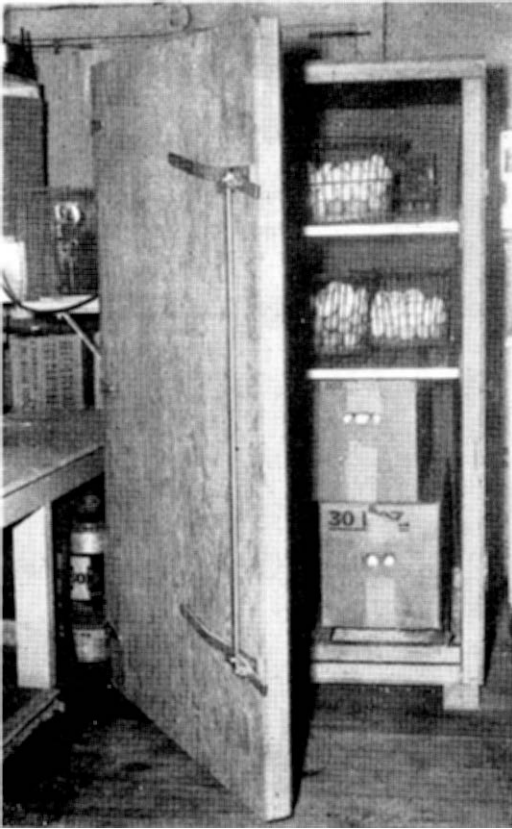
Figure 3. Shop-built, 7 case egg cooler used in experiments.
