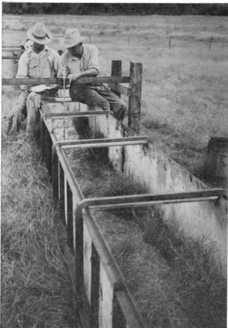
Figure 6.—Taking point gage measurements across the surface of the water. Note that the Bermuda grass is not completely submerged by this flow, which is approximately six inches deep.
