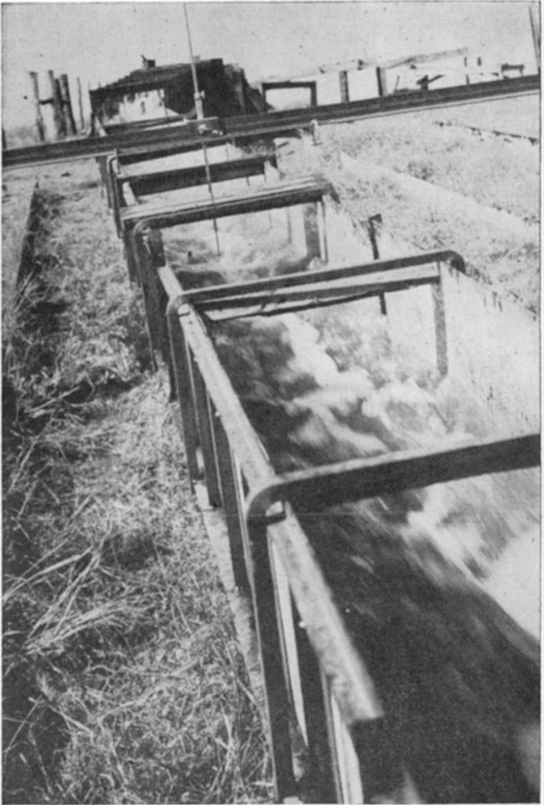
Figure 5. —A very turbulent flow at about 11 feet per second down a 10 percent slope. Note point gage mount and movable duct used to connect upper end of the channel to the concrete forebay.
