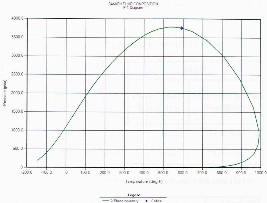
Figure 4.6: Pressure-Temperature diagram displaying 2 phase envelope for the representative fluid (WINPROP™)
