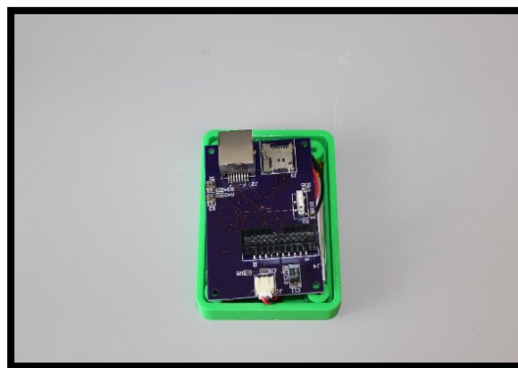
Figure 8.5.2: Bottom piece w battery & PCB
