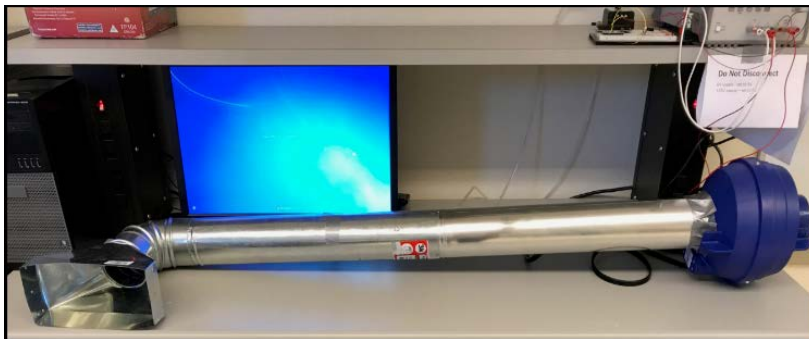
Figure 6.1.1: Airflow sensor test fixture
