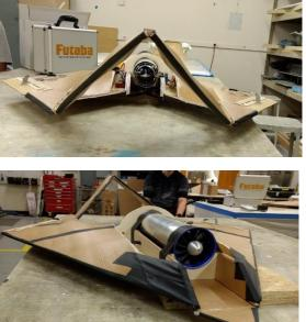
Flight of the foamies validated the CFD data and showed that the aircraft was remarkably stable in yaw, had little to no wing rock, and was capable of spot landing.
