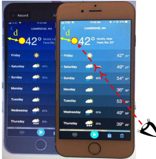
Figure 14. Experimental setup showing an example of how a user's eye fixation (yellow circle) on the actual smartphone appear on the emulated interface with the same distance (d) from a reference point
