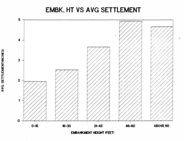
Fig. 7 Settlement vs. approach embankment height relationship.
