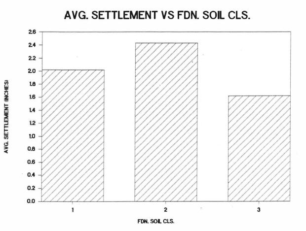
Fig. 8 Settlement vs. foundation soil type relationship.
