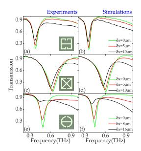
FIG. 4. (Color online) Measured (a) and simulated (b) amplitude transmission spectra of the capacitor-enhanced double SRRs with varying asymmetry. [(c) and (d)] show the measured and simulated spectra of the crossed double SRRs. [(e) and (f)] show the measured and simulated spectra of the circular double SRRs.
