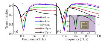
FIG. 2. (Color online) Measured (a) and simulated (b) amplitude transmission spectra of the rectangular double SRRs with varying asymmetry. The inset of (b) shows transmission spectra of the equidirectional displaced rectangular SRRs with  $\delta x$ =0,8,16  $\mu$ m, respectively.
