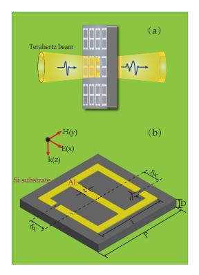
FIG. 1. (Color online) (a) Experimental configuration for the terahertz transmission measurements of a periodic array of planar metamaterials. (b) Schematic of the rectangular double SRR unit cell and the silicon substrate with a minimum feature  $d=3 \ \mu$ m in the splits of the rings and other structural dimensions  $t=5 \ \mu$ m,  $l=50 \ \mu$ m, and a lattice periodicity  $P=65 \ \mu$ m.
