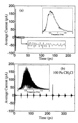
FIG. 2. (a) THz reference pulse for evacuated cell. Lower inset is time response of residual water vapor. The spectral response of the system is shown in the upper inset; spectral features result from result from residual water vapor. (b) Reshaped THz pulse and subsequent train of coherent transients with 100 Pa of methyl chloride.
