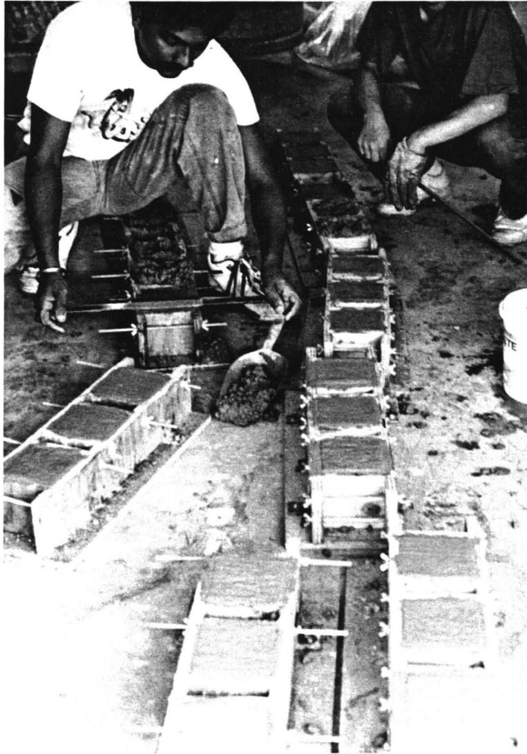
Fig. 3.6 Specimen Casting, NCHRP 244 Cubes
