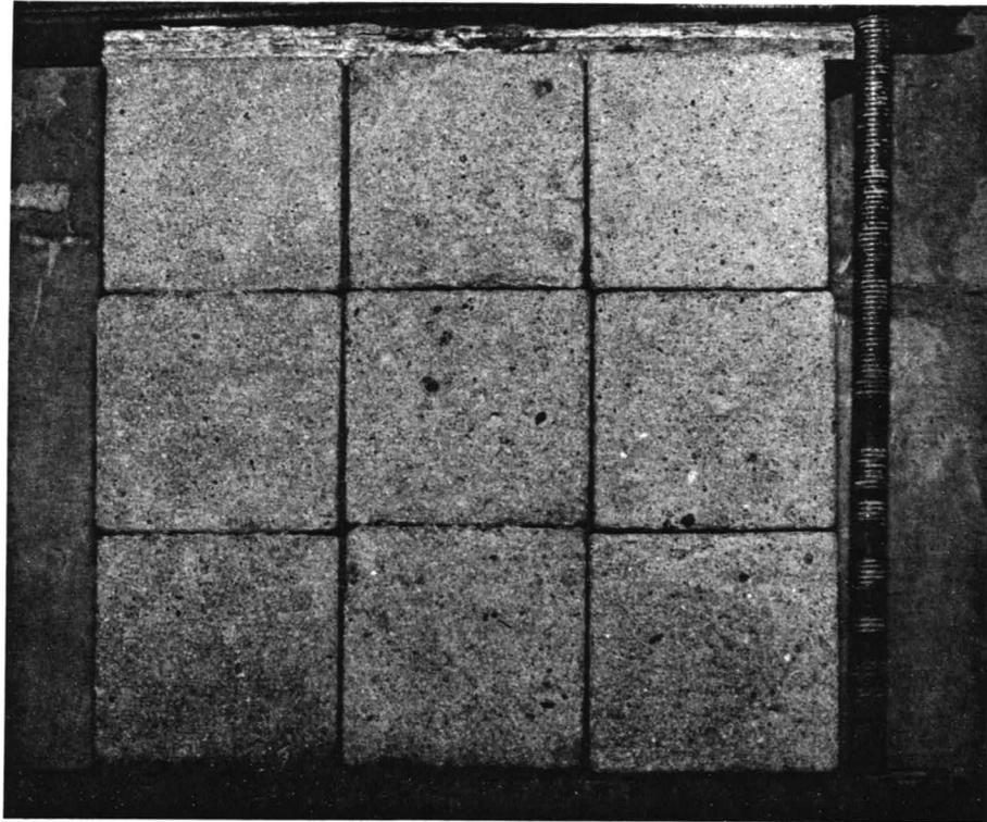
Fig. 3.10 Phase III Cubes After Shot-Blasting
