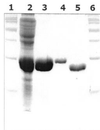
FIG. 3. SDS-12.5% polyacrylamide gel showing steps involved in purification of B. anthracis Sterne rDHFR. Lanes 1 and 6 contain Novagen Perfect Protein markers (15 to 150 kDa ladder). Lane 2 contains cell lysate from E. coli BL21 Star (DE3) carrying plasmids pLysS and pCRT7/CT-TOPO-Sterne rDHFR with the six-histidine tag (precolumn) (lysate filtered through a 0.22- \mu\text{m} -pore-size filter). Lane 3 contains pooled Sterne rDHFR with the six-His tag (enzyme purified by passage through a nickel column). Lane 4 contains FPLC-purified Sterne rDHFR with the six-His tag, and lane 5 contains FPLC-purified Sterne rDHFR with the six-His tag removed.
